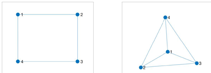
Figure 10: Graph structures for the electronic implementation of the network connection of N = 4 non-identical nodes. In the left a nearest neighbor connection and in the right a fully connected network.
