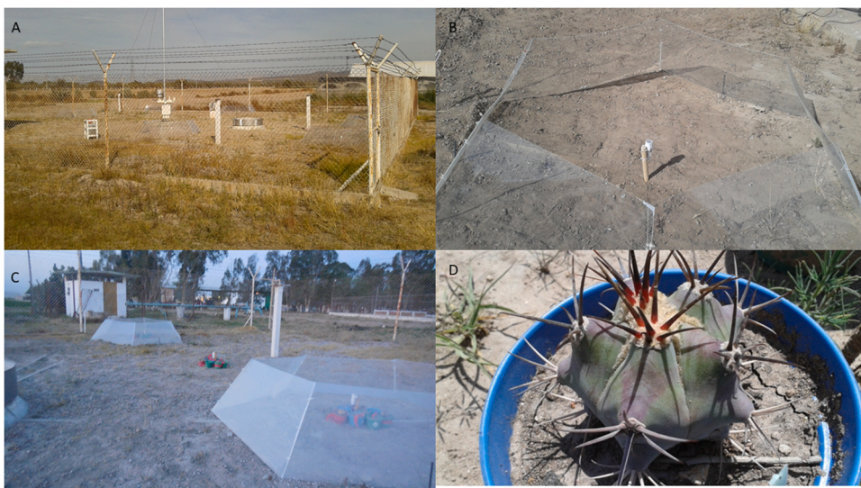
Fig. 1. Section of abandoned agricultural field used to induce global warming in the municipality of Soledad de Graciano Sanchez, San Luis Potosí, Mexico. A) Experimental site, B) Example of hexagonal open top-chamber (OTC) used to simulate the effects of global warming, C) Experimental design showing open top-chambers (OTC) and control plots, and D) Five-years old individuals of Echinocactus platyacanthus .
