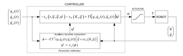
Figure 3.4: Block diagram of the proposed adaptive control scheme
