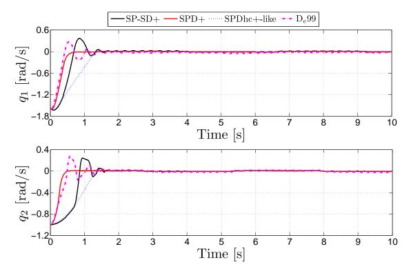
Figure 5.14: Test 2: position errors
