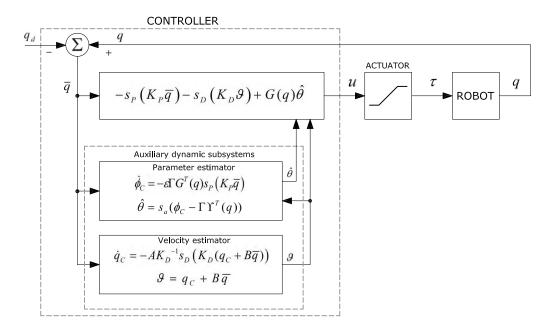
Figure 3.2: Block diagram of the output-feedback adaptive scheme
