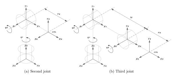
Figure A.3: Frame placement to compute the Jacobian of each joint
