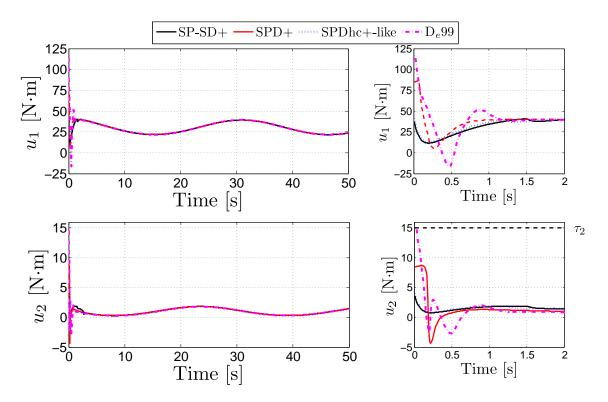
Figure 4.19: Test 2: control signals
