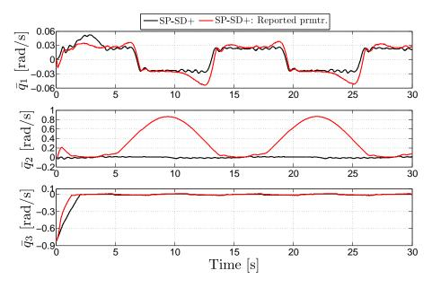
Figure 5.31: Test 2: Position errors of the SPSD+ scheme
