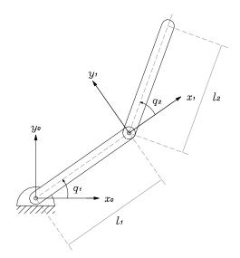
Figure A.1: 2 DOF Robot Manipulator
