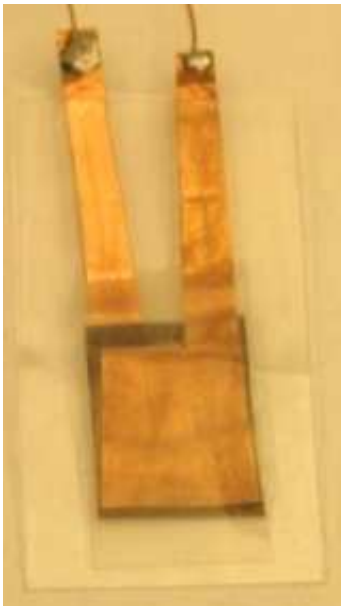
Figure 2.4: Photograph of the gold coated piezo-paper placed between two copper foils for current collection.
