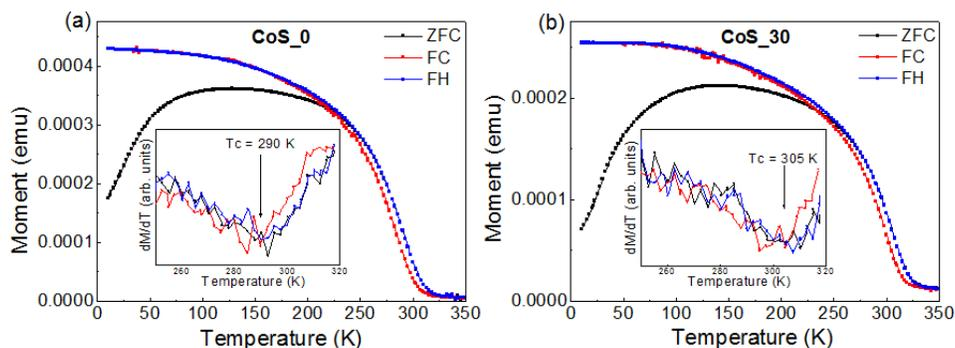
Fig. 4. ZFC, FC and FH  $M(T)$  curves measured under a constant applied magnetic field of 50 mT for CoS<sub>0</sub> and CoS<sub>30</sub> co-sputtered films. Inset:  $dM/dT$  vs.  $T$  curve
