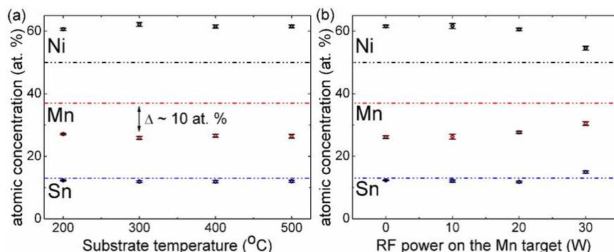
**Fig. 1. Calculated average atomic concentration and standard deviation for Ni, Mn and Sn elements of the sputtered (a) and co-sputtered (b) films. the horizontal dashed straight lines in the graphs represent the target elemental atomic composition Ni:Mn:Sn = 50:37:13**
