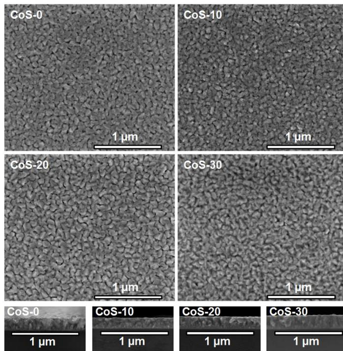
Fig. 3. SEM micrographs of the film surface and cross-sectional granular structure of CoS<sub>0</sub>, CoS<sub>10</sub>, CoS<sub>20</sub>, and CoS<sub>30</sub> co-sputtered films
