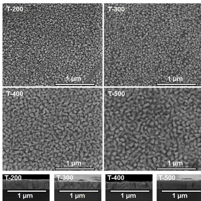
**Fig. 2. SEM micrographs of the film surface and cross-sectional granular structure of T\_200, T\_300, T\_400 and T\_500 sputtered films**
