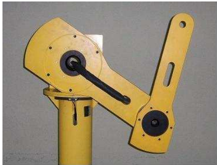
Fig. 1: Experimental setup: 2-DOF revolute-joint mechanical manipulator
