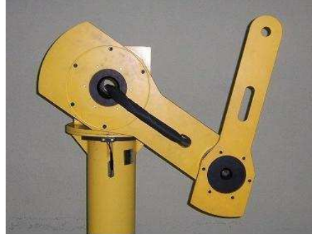
Fig. 2. Experimental setup: 2-DOF direct-drive robot manipulator
