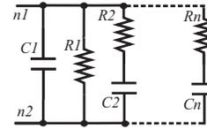
Fig. 3. Fractance device of  $1/s^\alpha$ .
