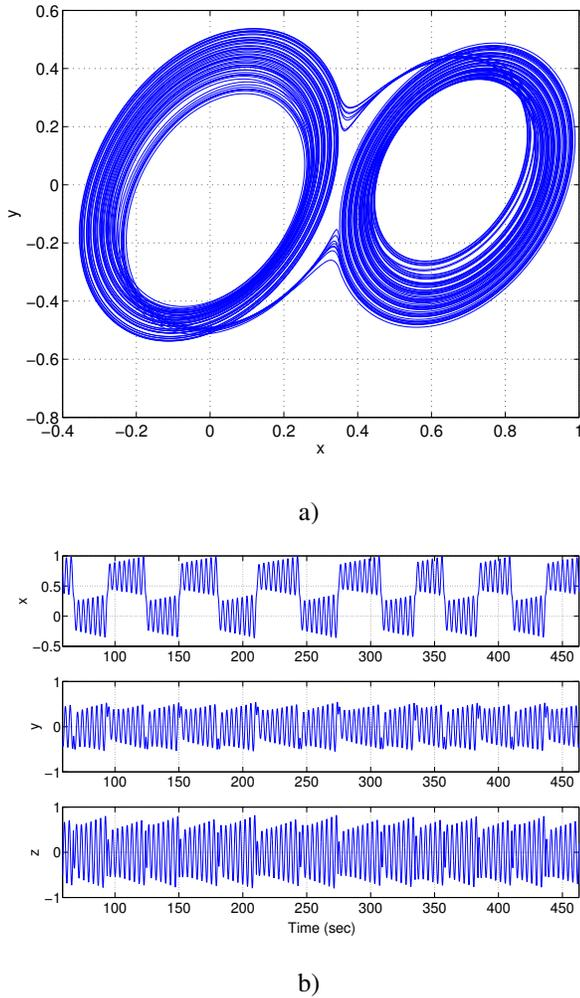
Fig. 1. a) Projections of the attractors onto the  $xy$ -plane. b) Chaotic signals of the fractional order chaotic system against to time.
