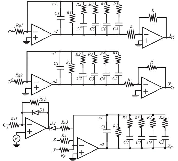
Fig. 4. Circuit diagram to realize the fractional order unstable dissipative system (11) for  $\alpha = 0.8$ .
