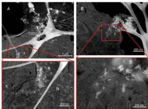
Figure 3.13 STEM image of HeLa cells treated with f COx-MWNT. Some nanotubes in figure A cross the cell membrane and nucleus. In B it appears that the cell phagocytoses CNTs, thus avoiding cell damage. Nanotube concentration correspond to 10 \mu\text{g ml}^{-1}
