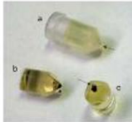
Figure 3.3. Embedded cells into epoxy resin. Figure a shows the capsule-mold having a trapezoidal shape on the tip. In figures b and c we can observe the trapezoidal shape. Arrows indicate the cellular sample located close to the tip of the capsule.
