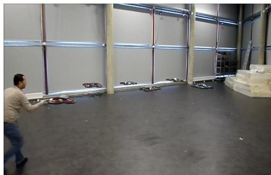
Fig. 14: Experiment with pull perturbation
