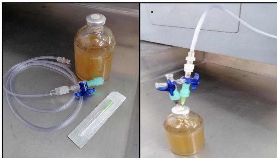
Fig. 3. Headspace exchange on the serum bottles.
