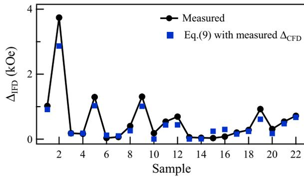
**Figure 6.** Interaction field distribution width,  $\Delta_{\text{IFD}}$ , measured from the FORC diagrams (line with circles) compared with the width calculated with Eq. (9) using the measured values of  $\Delta_{\text{CFD}}$  and  $H_c$  (squares).
