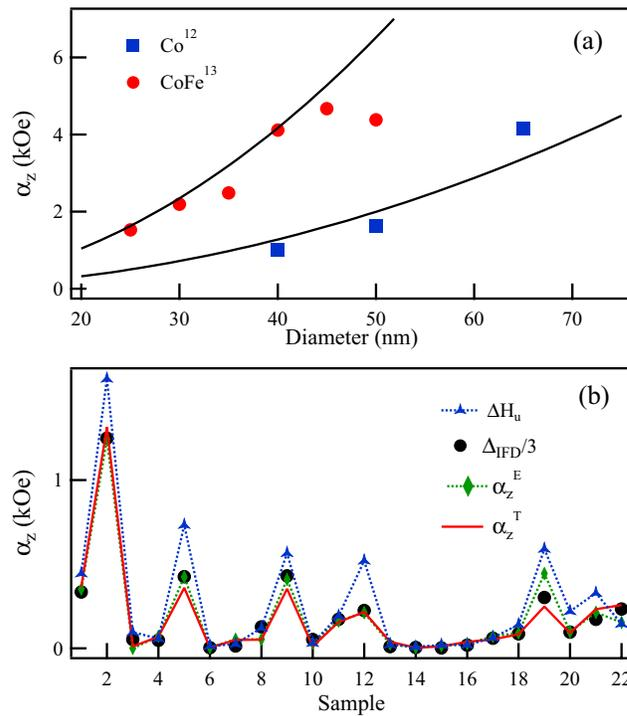
**Figure 3.** Interaction field coefficient,  $\alpha_z$  (a) calculated using Eq. (4) for Co and CoFe NWs (continuous lines) compared to the experimental values of  $\Delta H_u$  reported in Refs.<sup>12,13</sup>, and (b) Comparison of the values of  $\Delta H_u$  and  $\Delta_{IFD}/3$  measured from the FORC diagrams and the experimental ( $\alpha_z^E$ ) as well as theoretical ( $\alpha_z^T$ ) values of the axial component of the magnetization dependent interaction field.
