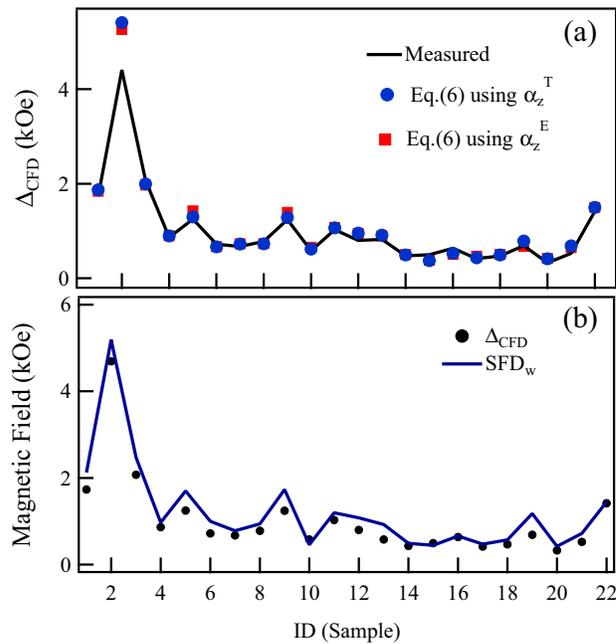
**Figure 4.** (a) Coercive field distribution width,  $\Delta_{CFD}$ , measured from the FORC diagrams (continuous line) compared with the width calculated with Eq. (6) using the theoretical (circles) and experimental values (squares) of  $\alpha_z$ , and (b) Comparison between the full width of the FORC-CFD,  $\Delta_{CFD}$  and the full width of the SFD,  $SFD_w$  obtained by derivation of the major DCD remanence curve.
