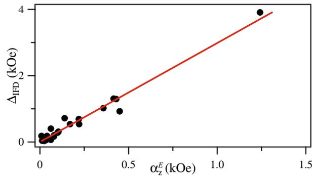
**Figure 2.** Measured width of the IFD distribution,  $\Delta_{\text{IFD}}$ , plotted as a function of the axial component of the interaction field  $\alpha_z^E$  measured from the IRM/DCD remanence curves. The straight line corresponds to the fit of  $\Delta_{\text{IFD}} = 3\alpha_z$ .
