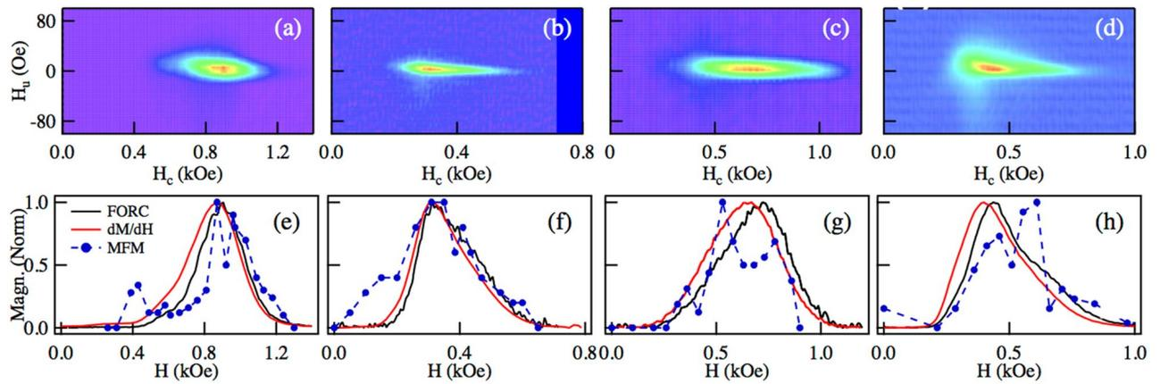
**Figure 5.** FORC diagram measured in low packing fraction ( $P = 0.4\%$ ) NWs, (a) 50 nm CoFe [S13], (b) 71 nm NiFe [S15], (c) 50 nm Ni [S6], and (d) 71 nm CoFe [S16]. The corresponding CFDs measured using the FORC diagram, the SFD ( $dM/dH$ ) and MFM are shown in (e)–(h), respectively.
