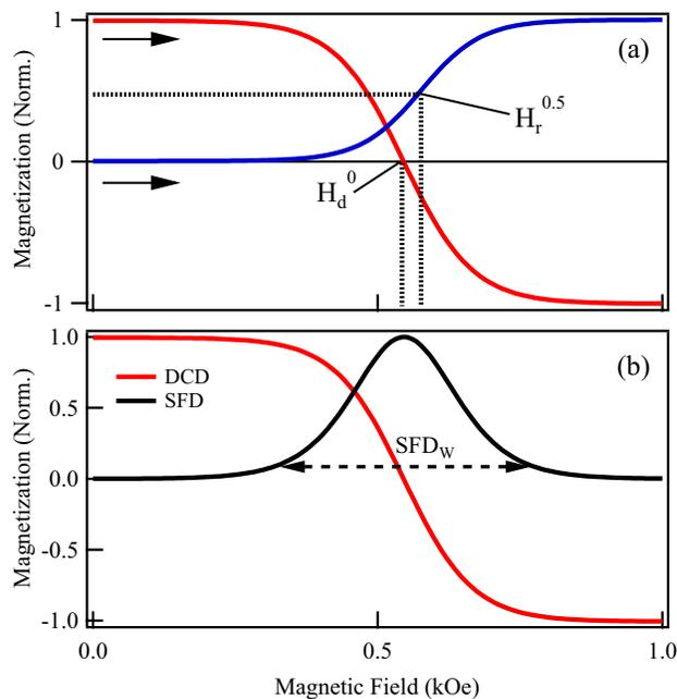
**Figure 7.** (a) Typical IRM and DCD remanence curves. The field value at which the normalized IRM curve is equal to 0.5,  $H_r^{0.5}$ , and the field value at which the DCD curve is zero  $H_d^0$  are indicated. The arrows indicate the field sweep sense. (b) The DCD remanence curve and its derivative (SFD), where the maximum width,  $SFD_w$  is indicated.
