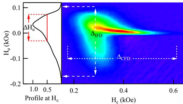
**Figure 1.** FORC diagram plotted in the  $H_c$ ,  $H_u$  plane measured for the sample S17 (Ni,  $\phi=100\text{nm}$ ,  $P=2.0\%$ ), where the measured quantities are indicated: the interaction field distribution  $\Delta_{\text{IFD}}$ , the coercive field distribution  $\Delta_{\text{CFD}}$  and  $\Delta H_u$ .
