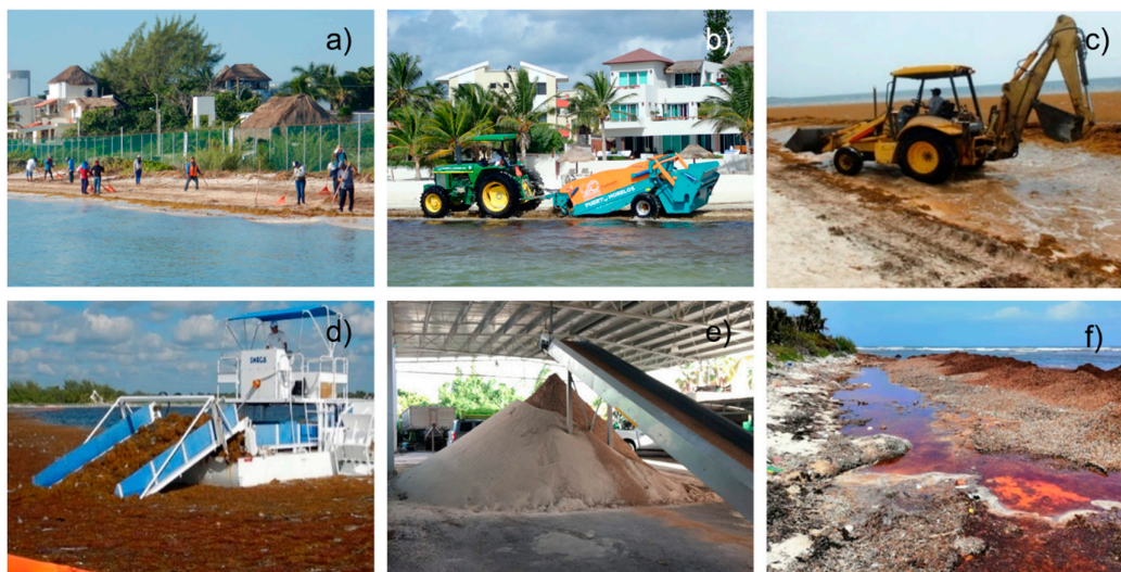
Figure 10. Removing beached sargasso from the Mexican Caribbean: (a–c) on the beach, and (d) in coastal waters. (e) Sand recovery in one of the hotels (huge amounts of sand are removed during sargasso clean-up activities on the beaches). (f) When large amounts of sargasso are left on the beach pools of leachates can be produced.
