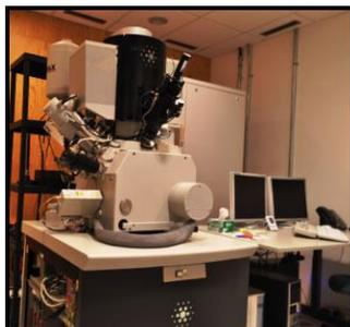
**Figura 4.3** FEI modelo FIB Dual Beam Helios Nanolab 600.
