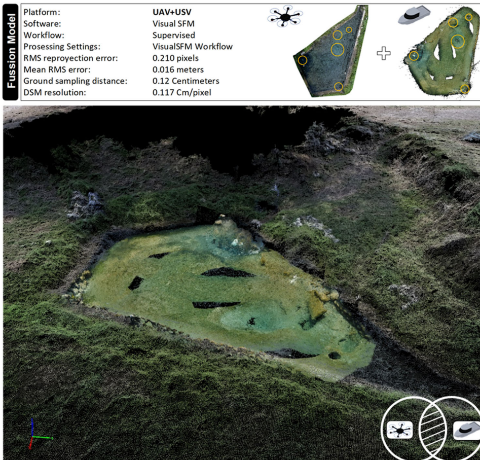
Figure 13. 3D reconstruction of data fusion from the platform used (UAV-USV).
