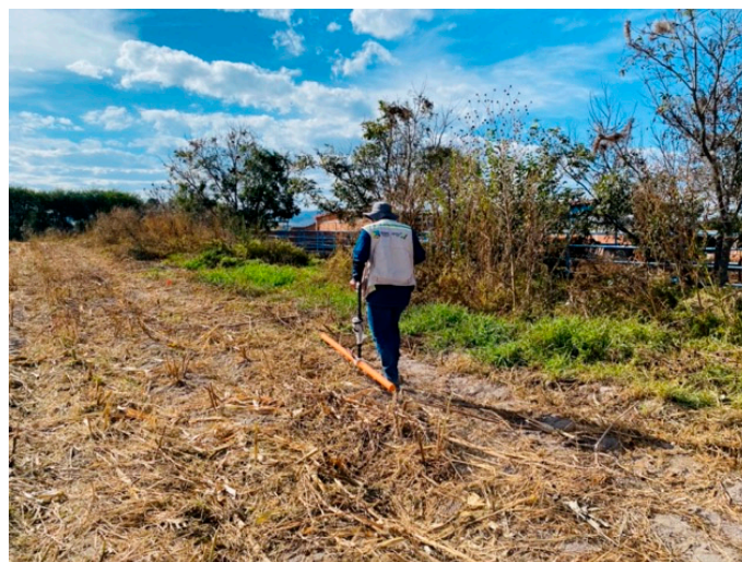
Figure 3. Electrical conductivity survey using the EMP meter on route or on profile.
