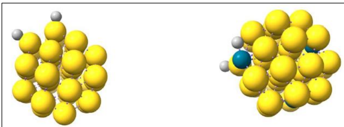
Figure 3-9. Optimized geometries of Au 38 -H 2 and Au 34 Pd 4 -H 2 clusters at the DFT/PBE-D3BJ level. Colors: Au in yellow, Pd in turquoise blue, H in grey.
