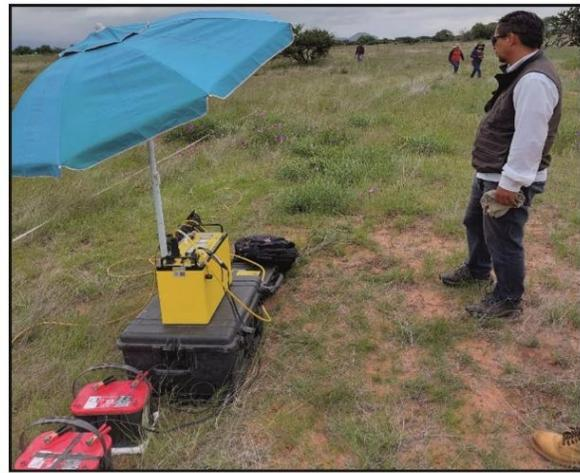
Fig. 5. SuperSting R8 multi-electrode resistivity meter.
