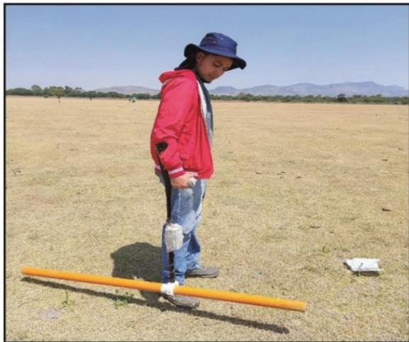
Fig. 4. CMD-MiniExplorer 6 I EM conductivity meter.
