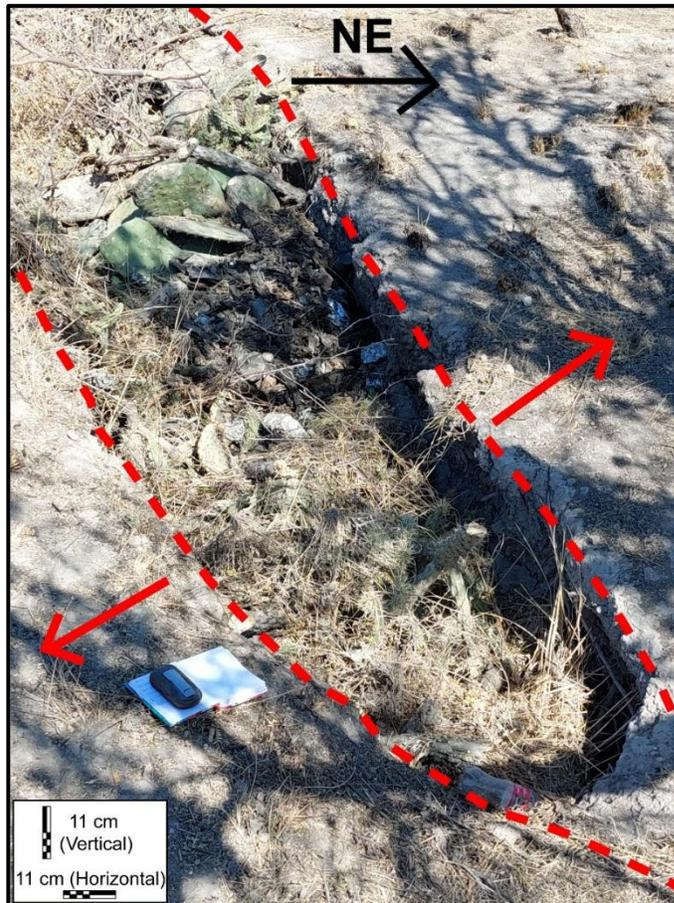
**Figure 13** Ground subsidence spots visible along the main fault trace.
