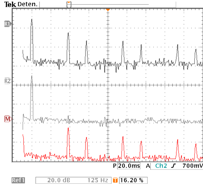
Fig. 7.4: Frequency spectrum of (from top to bottom) the load current i_L , fundamental component i_{Lf} , and harmonic component i_{Lh} . (x-axis 125Hz/div, y-axis 20 A/div).
