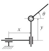
Figure 3.1: Schematic representation of the underactuated PPR manipulator of system (3.24).
