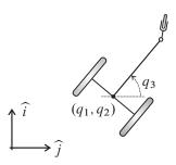
Figure 1.1: Schematic diagram of the unicycle-type wheeled robot of system (1.2).
