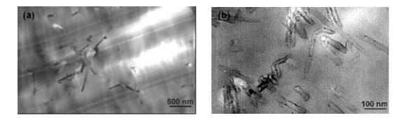
Fig. 6.8. TEM images of polymer nanocomposites of PS and 2 wt% of PS-grafted CN<sub>x</sub> nanotubes (PS-*g*-CN<sub>x</sub>) prepared by solution casting and high temperature pressing.
