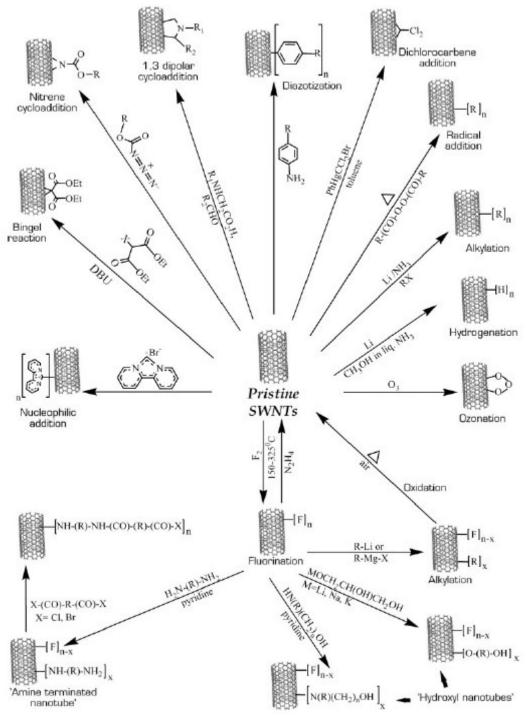
Fig. 2.7. Covalent-sidewall functionalization reactions of carbon nanotubes [1].
