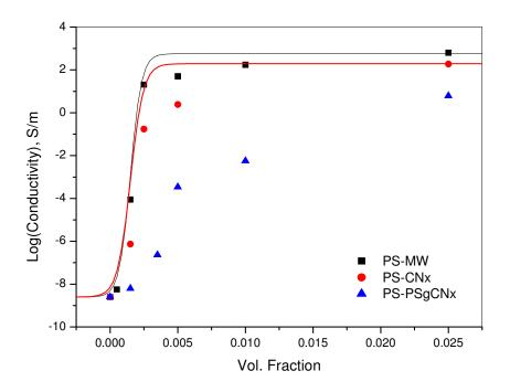
Fig. 7.31. Insulator-conductor transition model applied to PS/CNTs composites.
