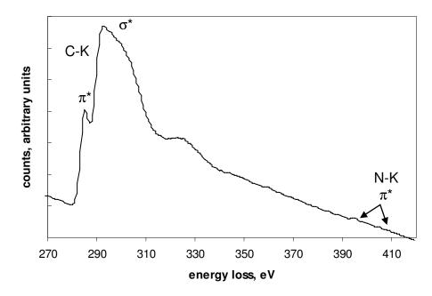
Fig. 4.3. Core-loss EEL spectra of the as prepared-CN<sub>x</sub> nanotubes, showing the C and N edges.
