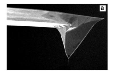
Fig. 1.16. SEM image of a standard AFM tip with a MWNT attached.
