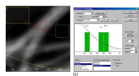
Fig. 5.11. EFTEM spectra extracted from the energy-filtered image series, sorted by element and the parameters used for the calculation of the elemental maps in CN<sub>x</sub>-RNO<sub>x</sub> (3):
