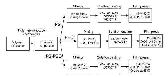
Fig. 6.1. Reaction scheme of the preparation steps of the polymer-nanotube composites.
