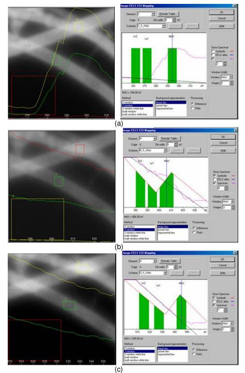
5.1. EFTEM spectra from the energy-filtered image series of CN<sub>x</sub> NTs
