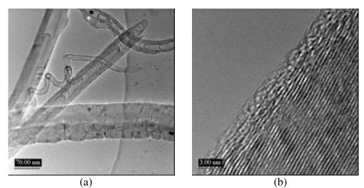
Fig. 4.2. HRTEM images of raw CN<sub>x</sub> nanotubes after sonication in ethanol: (a) overall view, (b) nanotube crystalline planes and carbon amorphous layer.
