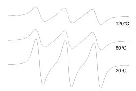
Fig. 5.15. EPR Spectra of PR CGX505 nitroxide recorded at several temperatures 20, 80 and 120°C in xylene as solvent.
