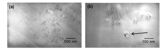
Fig. 6.6. TEM images of polymer nanocomposites of PS and 2 wt% of  $CN_x$  nanotubes prepared by solution casting and high temperature pressing.
