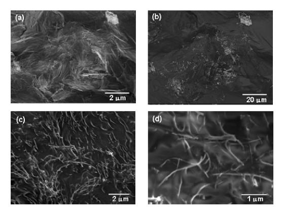
Fig. 6.14. SEM images of polymer nanocomposites of PEO and 2 wt% of  $CN_x$  nanotubes prepared by solution casting and film pressing. Images (a) and (c) taken at normal scan and (b) and (d) at slow scan.
