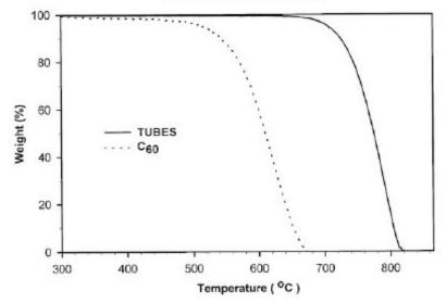
Fig. 1.10. Thermogravimetric Analysis of a MWNTs and  $C_{60}$ . As can be seen the nanotubes are more resistant than  $C_{60}$  to oxidation processes [2].
