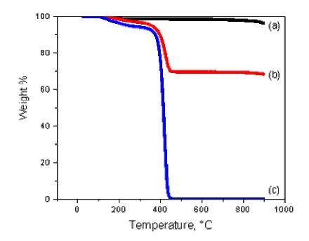
Fig. 5.19. Thermal degradation of reaction products of *in situ* polymerized  $CN_x$  nanotubes using BPO/PR CGX 505 (reactor F3), separated by filtration: (a) as-produced  $CN_x$  nanotubes, (b) over filter sample, corresponding to the PS-grafted from radical functionalized  $CN_x$  nanotubes, and (c) under filter sample, corresponding to PS.
