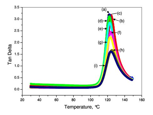
Fig. 7.14. Tan  $\delta$  of PS/PS-*g*-CN<sub>x</sub> nanocomposites vs. temperature at filler weight fractions of (a) 0, (b) 0.1, (c) 0.3, (d) 0.5, (e) 0.7, (f) 1.0, (g) 2.0, (h) 5.0, and (i) 7.7 wt%.
