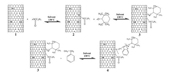
Fig. 4.6. Polymer brushes reaction scheme: functionalization of  $CN_x$  nanotubes (1) with the NMRP initiator (2) and controller (3), and synthesis of polymer brushes of polystyrene (4).
