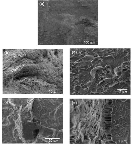
Fig. 6.22. SEM images of polymer nanocomposites of PS and PEO blends (35:65 wt%) and 2 wt% of polymer grafted nanotubes (PS-g-CN<sub>x</sub>).
