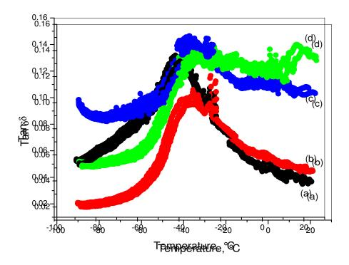
Fig. 7.28. Comparison of the Tan  $\delta$  of (a) PEO and PEO-based composite with (b) MWNT, (c) CN<sub>x</sub> and (d) PS-g-CN<sub>x</sub> nanotubes at a concentration of 2.0 wt%.
