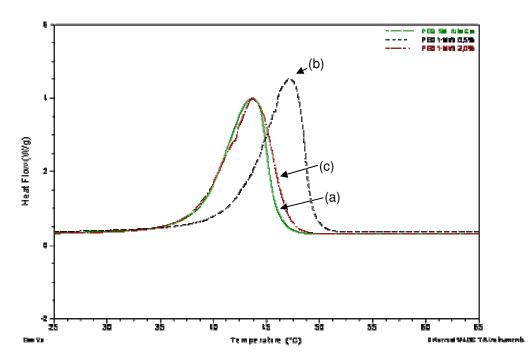
Fig. 6.12. Crystallization temperature of (a) PEO polymer matrix, and PEO/MWNT nanocomposites at several filler content: (b) 0.5 wt% and (c) 2.0 wt%.
