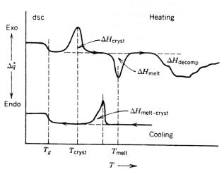
Fig. 4.16. Differential Scanning Calorimetry curve for a polymer which shows the glass transition temperature ( $T_g$ ), crystallization temperature ( $T_c$ ), melting temperature ( $T_m$ ), heat of crystallization ( $\Delta H_{cryst}$ ), heat of melting ( $\Delta H_{melt}$ ), heat of degradation ( $\Delta H_{decom}$ ) and heat of crystallization from the melt ( $\Delta H_{melt-cryst}$ ) [8].
