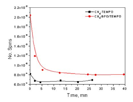
Fig. 5.16. Spin concentration as a function of time in samples of  $CN_x$  nanotubes and BPO/TEMPO radicals reacted in benzene at 105°C.
