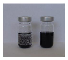
Fig. 5.18. Stability and solubility differences between (a) physical blend of PS and sonicated- $CN_x$  nanotubes, PS- $CN_x$ , (left hand side), and (b) *in situ* polymerized PS in the presence of radically functionalized  $CN_x$  (right hand side) in toluene. The former dispersion is not stable, whereas the second is stable over weeks.
