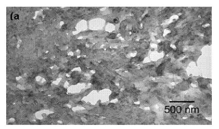
Fig. 6.21. TEM images of polymer nanocomposites of PS and PEO blends (35:65 wt%) and 2 wt% of CN<sub>x</sub> nanotubes.
