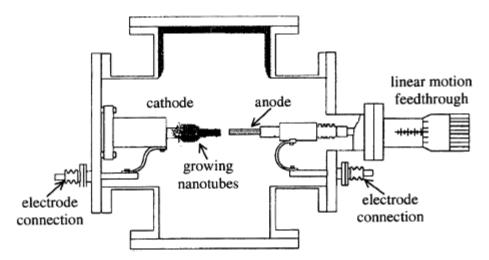
Fig. 1.5. Schematic representation of an electric-arc-discharge apparatus used to produce fullerenes and carbon nanotubes [18].
