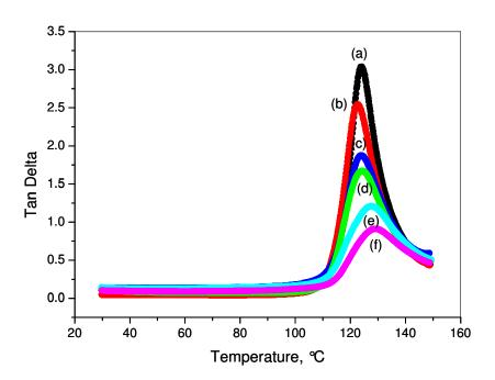
Fig. 7.10. Tan  $\delta$  of PS/MWNT nanocomposites vs. temperature at filler weight fractions of (a) 0, (b) 0.3, (c) 0.5, (d) 1.0, (e) 2.0 and (f) 5.0 wt%.
