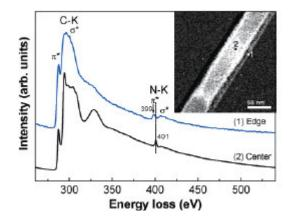
Fig. 1.11. EEL spectra of  $CN_x$  nanotube showing the C-K and N-K ionization edges for C and N at (1) the nanotube edge and (2) in the center of the nanotube [52].
