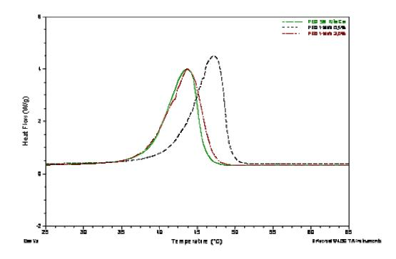
Fig. 6.17. Melting temperature of (a) pure PS-PEO polymer blend, and PS-PEO/MWNT nanocomposites at several filler content: (b) 0.5 wt% and (c) 2.0 wt%.
