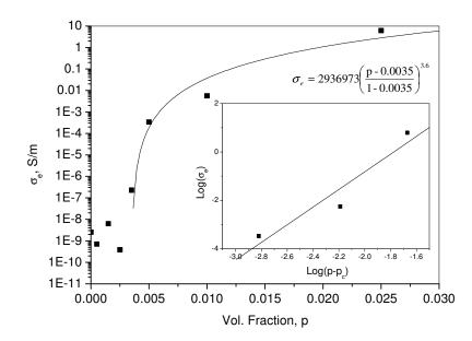
Fig. 7.34. Real part of the AC electrical conductivity at 1 Hz and applied voltage of 0.1 V for PS/PS-g-CN<sub>x</sub> at several filler contents. Comparison with statistical percolation theory (solid lines).
