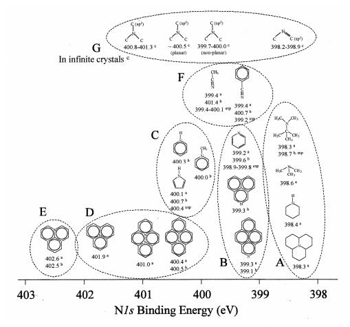
Fig. 1.13. Calculated N1s binding energy loss-near edge fine structures [55].
