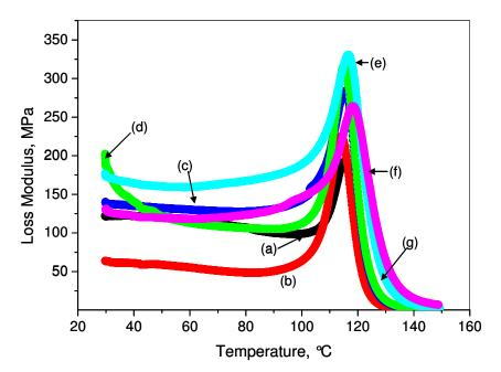
Fig. 7.9. Loss modulus of PS/MWNT nanocomposites vs. temperature at filler weight fractions of: (a) 0, (b) 0.3, (c) 0.5, (d) 1.0, (e) 2.0 and (f) 5.0 wt%.
