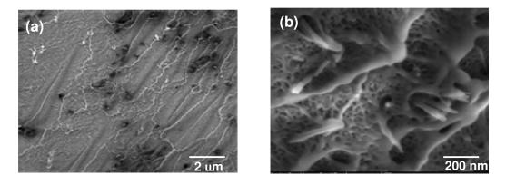
Fig. 6.5. SEM images of film fractured polymer nanocomposites of PS and 2 wt% of CN<sub>x</sub> nanotubes prepared by solution casting and high temperature pressing.
