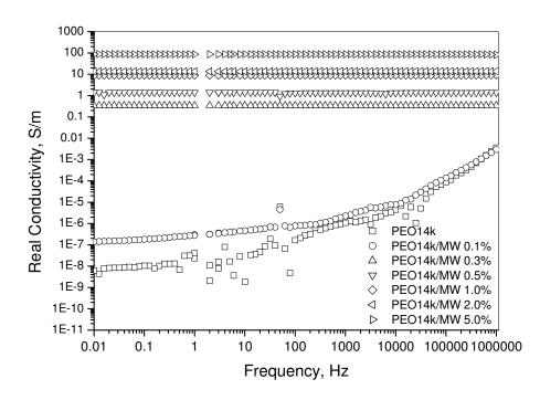
Fig. 7.41. Real conductivity of PEO14k/MWNT nanocomposites vs. frequency at filler weight fractions of 0.1 to 5.0 wt% and applied voltage of 0.1 V.
