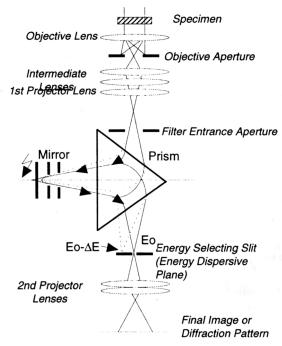
Fig. 4.8. Electron ray path of a Transmission Electron Microscope equipped with an in-column energy filter [6].
