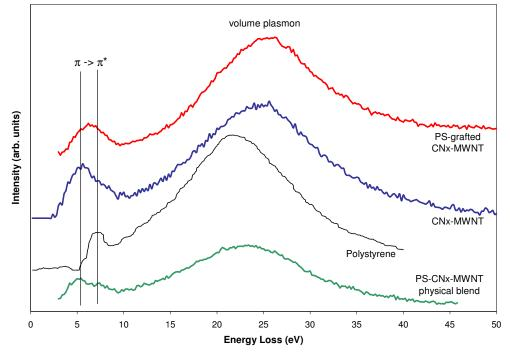
Fig. 5.24. EEL comparative spectra of the PS, raw  $CN_x$  nanotubes, PS-g- $CN_x$ , and the physical blend of PS and  $CN_x$  nanotubes.
