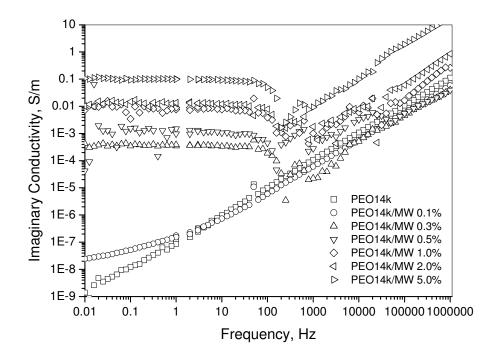
Fig. 7.42. Imaginary conductivity of PEO14k/MWNT nanocomposites vs. frequency at filler weight fractions of 0.1 to 5.0 wt% and applied voltage of 0.1 V.
