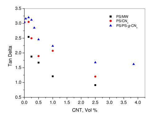
Fig. 7.15. Loss factor (tan  $\delta$ ) of the PS/CNTs composites at several volume fractions of: ( $\delta$ ) MWNT, ( $\Box$ ) CN<sub>x</sub> and ( $\circ$ ) PS-g-CN<sub>x</sub> nanotubes.
