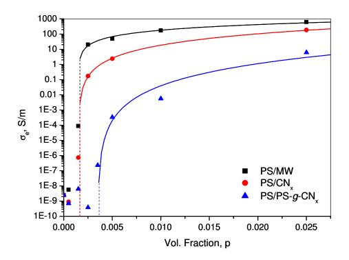
Fig. 7.7. Real part of the AC electrical conductivity at 1 Hz for nanocomposites of PS and nanotubes at several filler contents. Comparison with the statistical percolation theory (solid lines)
