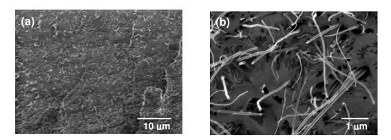
Fig. 6.3. SEM images of film-fractured polymer nanocomposites of PS and 2 wt% of MWNTs prepared by solution casting and high temperature pressing at several magnifications and scan velocities: (a) high scan, (b) low scan.
