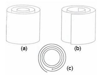
Fig. 1.4. Schematic representation of a) "Russian doll" and b) "Scroll-like" models for MWNTs [17]. A mixed configuration is also represented (c).
