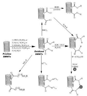
Fig. 2.6. Scheme of common covalent functionalization routes used to derive SWNTs at the ends and defect sites. As produced nanotubes are treated with an oxidative protocol to generate functional groups that react with SOCl<sub>2</sub> followed by amide or ester linkages. Amine and oxygenated functional groups are also effective sites for coordination to metal complexes and ions [1].
