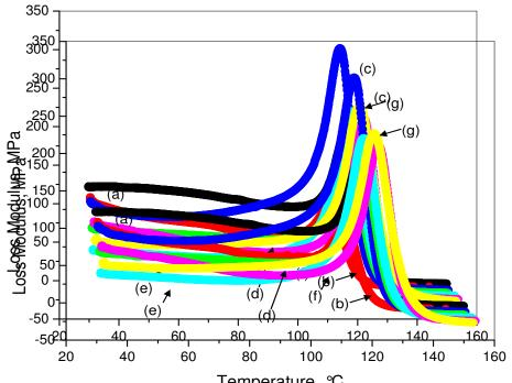
7.4. Loss modulus of PS/CNTs composites at several CNT concentration
