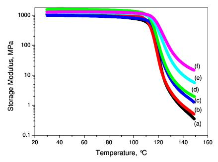
Fig. 7.8. Storage modulus of PS/MWNT nanocomposite vs. temperature at filler weight fractions of (a) 0, (b) 0.3, (c) 0.5, (d) 1.0, (e) 2.0 and (f) 5.0 wt%.
