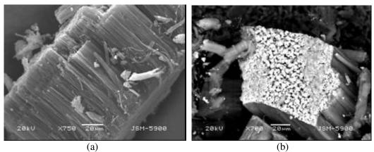
Fig. 4.1. SEM images of raw  $CN_x$  nanotubes: (a) nanotube bundles and (b) top-view of flakes showing the catalyst particles at the free ends of the nanotubes.
