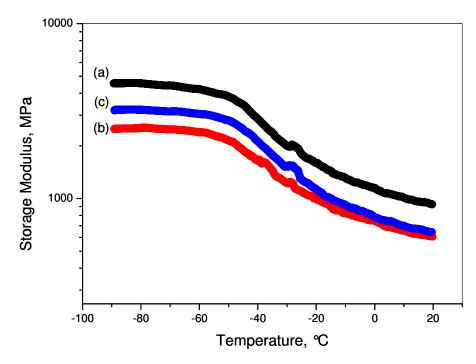
Fig. 7.25. Storage modulus of PEO/MWNT nanocomposite vs. temperature at filler weight fractions of (a) 0, (b) 0.5, and (c) 2.0 wt%.
