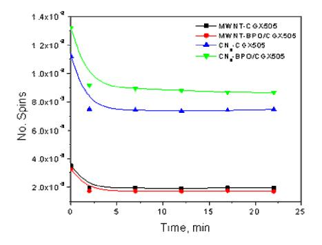
Fig. 5.17. Spin concentration as a function of time in samples of MWNT and CN<sub>x</sub> nanotubes with BPO/PR CGX505 radicals reacted in xylene at 120°C.
