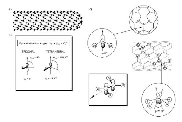
Fig. 2.1. Diagrams of (a) metallic (5,5) SWNT, (b) pyramidalization angle, and (c) misalignment angles ( $\phi$ ) along C1-C4 in the (5,5) SWNT and its capping fullerene C<sub>60</sub> [15].
