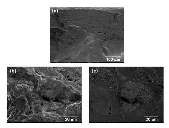
Fig. 6.19. SEM images of polymer nanocomposites of PS and PEO polymer blends (35:65 wt%) and 2 wt% MW nanotubes.
