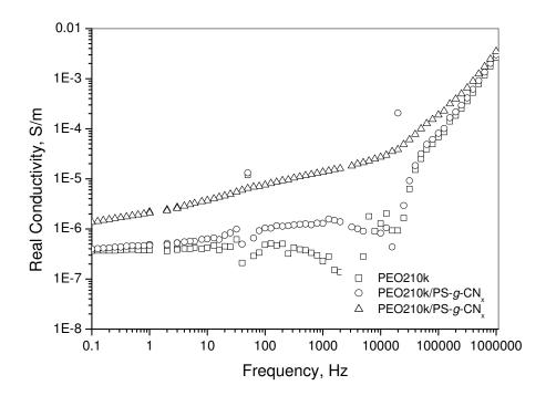
Fig. 7.23. Real conductivity of PEO210k/PS-g-CN<sub>x</sub> nanocomposites vs. frequency at filler weight fractions of 0.1 to 5.0 wt% and applied voltage of 0.1 V.
