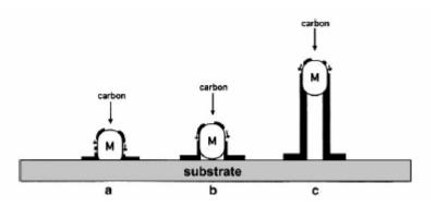
Fig. 1.20. Model representation of carbon nanotubes growth mechanism from a substrate by the carbon diffusion over the metal catalyst particle,M. Vertical fibers of graphite are formed between metal and substrate [14].
