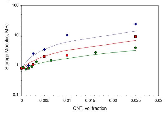
Fig. 7.19. Storage modulus of the PS/CNTs composites at several volume fractions of:
