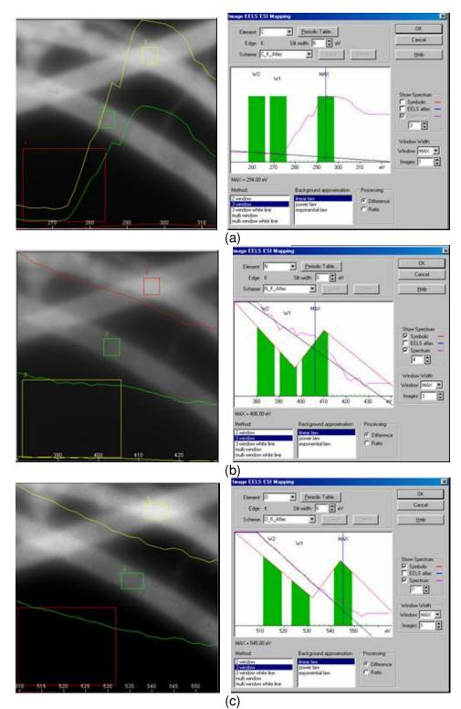
Fig. 5.10. EFTEM spectra extracted from the energy-filtered image series, sorted by element and the parameters used for the calculation of the elemental maps in  $CN_x$  nanotubes (1): (a) carbon map, (b) nitrogen map and (c) oxygen map.
