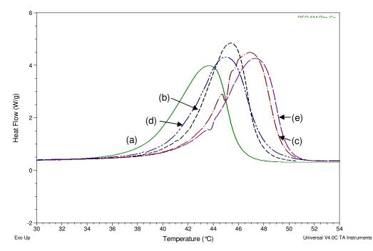
Fig. 6.11. Crystallization peak for (a) PEO polymer matrix, and PEO-based nanocomposites: PEO/CN<sub>x</sub> (b) with 0.5 wt%, and (c) with 2.0 wt%, PEO/PS-g-CN<sub>x</sub> (d) with 0.5 wt% and (e) with 2.0 wt%.
