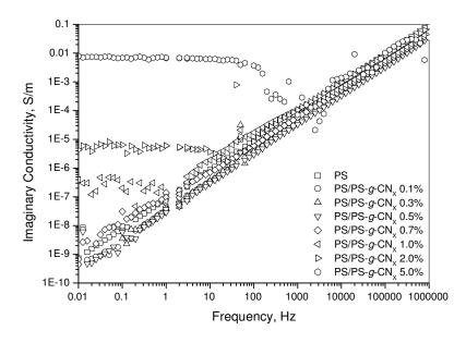
Fig. 7.30. Imaginary conductivity of PS/PS-*g*-CN<sub>x</sub> nanocomposites vs. frequency at filler weight fractions of 0.1 to 5.0 wt% and applied voltage of 0.1 V.
