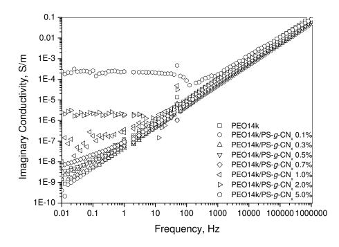
Fig. 7.46. Imaginary conductivity of PS-*g*- $CN_x$  nanocomposites vs. frequency at filler weight fractions of 0.1 to 5.0 wt% and applied voltage of 0.1 V.
