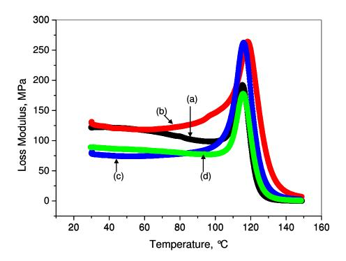
Fig. 7.37.Comparison of the loss modulus of (a) PS and PS-based composite with (b) MWNT, (c)  $CN_x$  and (d) PS-g-CN<sub>x</sub> nanotubes at a concentration of 5.0 wt%.
