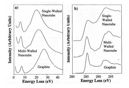
Fig. 4.9. Comparative EEL spectra of graphite, bundle of SWNTs and MWNTs in energy ranges of (a) 0 to 45 eV (plasmon region) and (b) 280-300 eV (carbon K-edge) [6].
