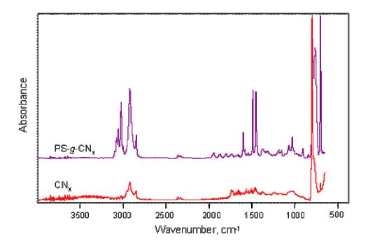
Fig. 5.29. FTIR spectra of CN<sub>x</sub> nanotubes and PS-g-CN<sub>x</sub> nanotubes.
