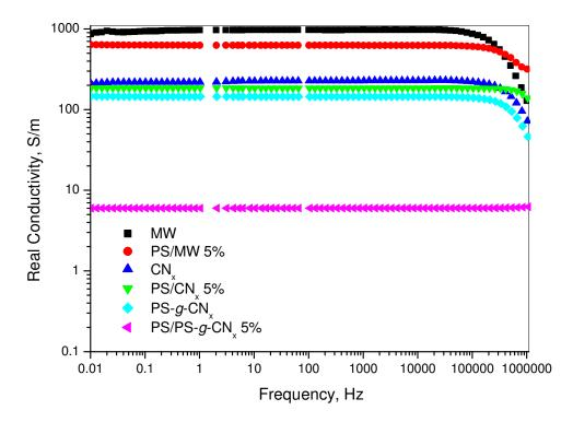
Fig. 7.1. Conductivity measures of several carbon nanotube fillers, and their correspondent PS-based nanocomposites filled at 5 wt% of filler.
