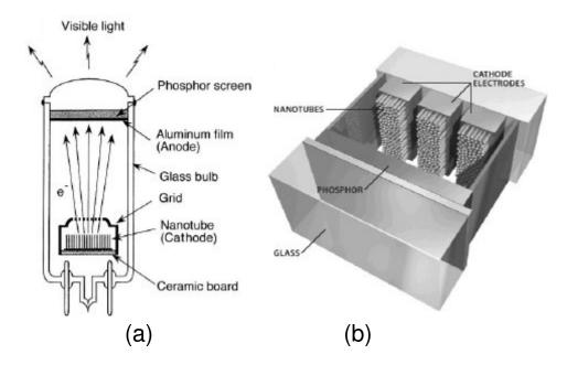
Fig. 1.14. Longitudinal cross-section of a fluorescent display with a field emission cathode constructed from MWNTs; (b) TV display prototype using CNTs [2].
