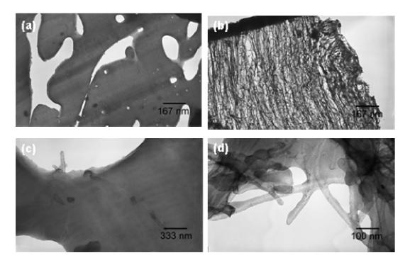
Fig. 6.23. TEM images of polymer nanocomposites of PS and PEO blends (35:65 wt%) and 2 wt% of polymer grafted nanotubes (PS-g-CN<sub>x</sub>) at several magnifications.
