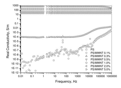
Fig. 7.3. Real conductivity of PS/MWNT nanocomposites vs. frequency at filler weight fractions of 0.1 to 5.0 wt% and applied voltage of 0.1 V.
