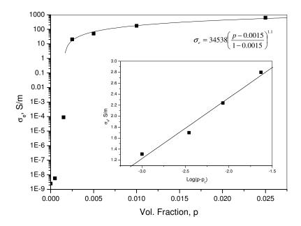
Fig. 7.32. Real part of the AC electrical conductivity at 1 Hz and applied voltage of 0.1 V for PS/MWNT at several filler contents. Comparison with statistical percolation theory (solid lines).
