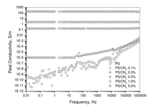
Fig. 7.5. Real conductivity of  $PS/CN_x$  nanocomposites vs. frequency at filler weight fractions of 0.1 to 5.0 wt% and applied voltage 0.1 V.
