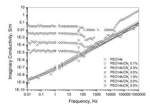
Fig. 7.44. Imaginary conductivity of PEO14k/CN<sub>x</sub> nanocomposites vs. frequency at filler weight fractions of 0.1 to 5.0 wt% and applied voltage of 0.1 V.
