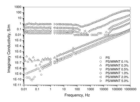
Fig. 7.4. Imaginary conductivity of PS/MWNT nanocomposites vs. frequency at filler weight fractions of 0.1 to 5.0 wt% and applied voltage of 0.1 V.
