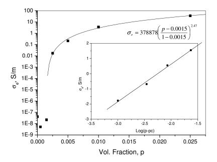
Fig. 7.48. Real part of the AC electrical conductivity at 1 Hz and applied voltage of 0.1 V for PEO14k/CN<sub>x</sub> composites at several filler contents. Comparison with model (solid lines).
