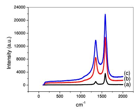
Fig. 5.14. Raman spectra of (a)  $CN_x$  nanotubes, and radical functionalized  $CN_x$  nanotubes with: (b) BPO/TEMPO and (c) BPO/PR CGX505 solutions.
