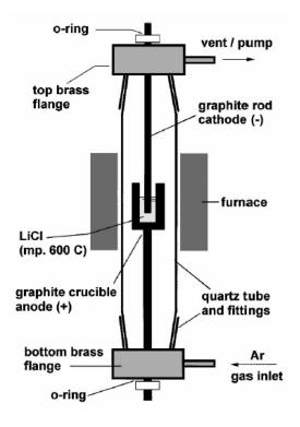
Fig. 1.8. Experimental set up of the electrolysis method used to synthesize CNTs in liquid phase [2].
