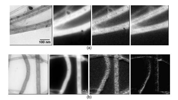
Fig. 5.26. Filtered images of (a)  $PS-g-CN_x$  and (b) physical blend of PS and  $CN_x$  nanotubes. Each group of images is presented in the next order: zero loss, carbon. nitrogen and oxygen maps.
