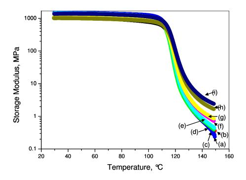
Fig. 7.13. Storage modulus of PS/PS-g-CN<sub>x</sub> nanocomposites vs. temperature at filler weight fractions of 0.1 to 5.0 wt%.
