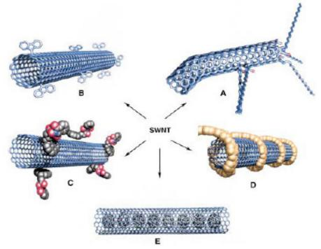
Fig. 2.5. Some functionalization possibilities of SWNTs: (A) Defect-group functionalization, B) covalent sidewall functionalization, (C) non-covalent exohedral functionalization with surfactants, (D) non-covalent exohedral functionalization with polymers, and (E) endohedral functionalization with, for example, C<sub>60</sub> [4].
