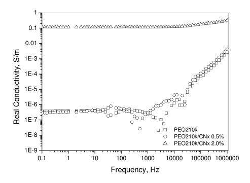
Fig. 7.22. Real conductivity of PEO210k/CN<sub>x</sub> nanocomposites vs. frequency at filler weight fractions of 0.1 to 5.0 wt% and applied voltage of 0.1 V.
