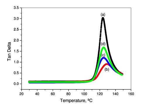
Fig. 7.18. Comparison of the Tan  $\delta$  of (a) PS and PS-based composite with (b) MWNT, (c)  $CN_x$  and (d) PS-g-CN<sub>x</sub> nanotubes at a concentration of 5.0 wt%.
