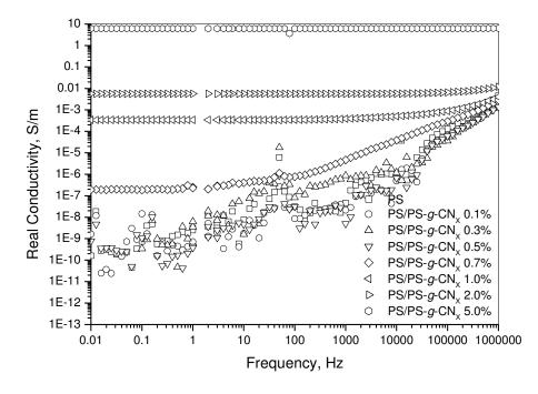
Fig. 7.6. Real conductivity of PS/PS-g-CN<sub>x</sub> nanocomposites vs. frequency at filler weight fractions of 0.1 to 7.7 wt% and applied voltage 0.1 V.
