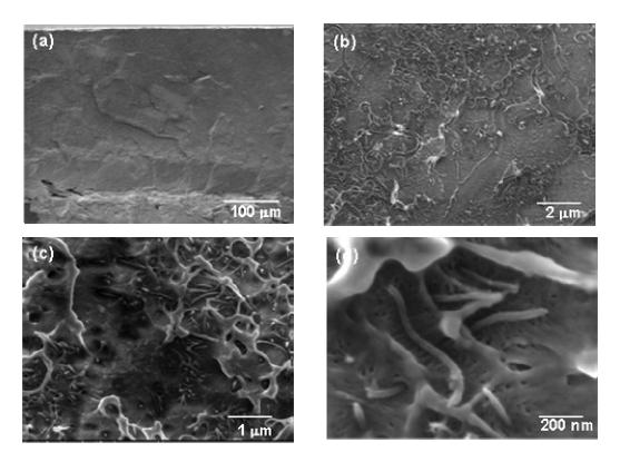
Fig. 6.7. SEM images of polymer nanocomposites of PS and 2 wt% of PS-grafted CN<sub>x</sub> nanotubes (PS-*g*-CN<sub>x</sub>) prepared by solution casting and high temperature pressing.
