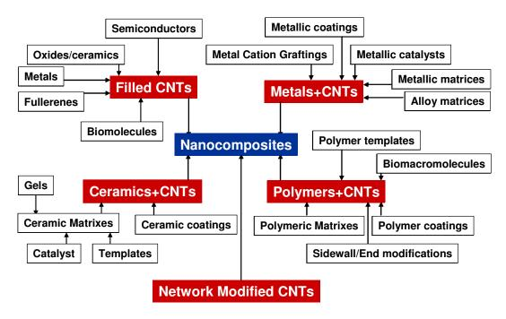
Fig. 3.1. Types of nanocomposites prepared using carbon nanotubes [7].
