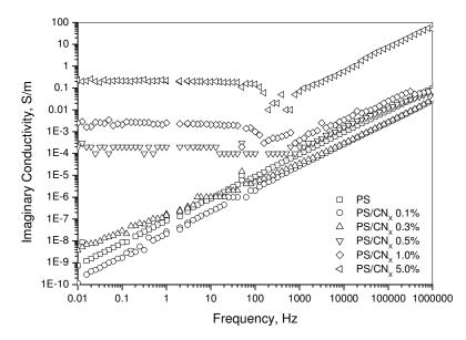
Fig. 7.29. Imaginary conductivity of PS/CN<sub>x</sub> nanocomposites vs. frequency at filler weight fractions of 0.1 to 5.0 wt% and applied voltage of 0.1 V.
