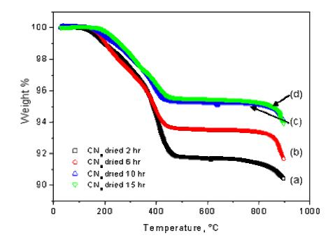
Fig. 5.3. Effect of the dried time in thermal degradation of  $CN_x$  sonicated in xylene (1 hr) and dried for (a) 2, (b) 6, (c)10 and (d) 15 hr in a vacuum oven at 70-80°C. TGA in N from 20-900°C at 10°C/min.
