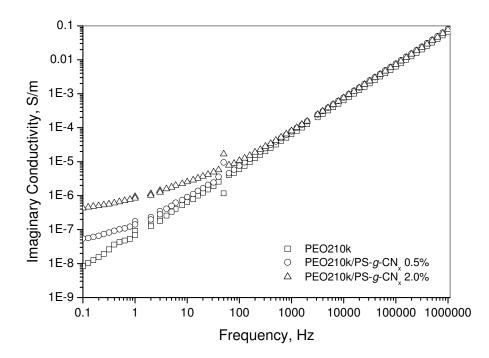
Fig. 7.40. Imaginary conductivity of PEO210k/PS-g-CN<sub>x</sub> nanocomposites vs. frequency at filler weight fractions of 0.1 to 5.0 wt% and applied voltage of 0.1 V.
