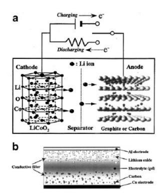
Fig. 1.15. (a) Charging-discharging mechanism of a Li battery; (b) basic composition of electrode and polymer Li+ composite of the battery [2].
