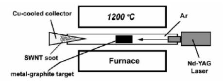
Fig. 1.6. Representation of the laser vaporization method to produce SWNTs and MWNTs. In this particular case the process is carried out in a furnace and the nanotubes are collected in a Cu-cooled trap [2].
