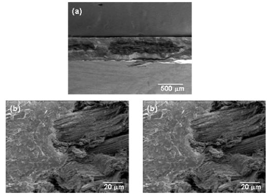
Fig. 6.20. SEM images of polymer nanocomposites of PS and PEO polymer blends (35:65 wt%) and 2 wt%  $CN_x$  nanotubes.
