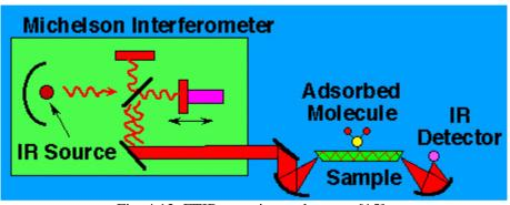
Fig. 4.12. FTIR experimental set up. [15]
