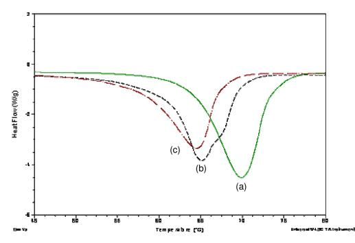
Fig. 6.9. Melting temperature of (a) PEO polymer matrix, and PEO/MWNT nanocomposites at several filler contents: (b) 0.5 wt% and (c) 2.0 wt%.
