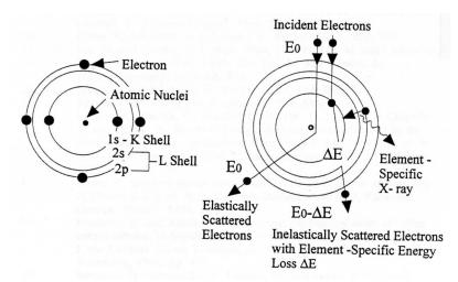
Fig. 4.7. Elastic and Inelastic Interactions between incident electron beam and atom [6].
