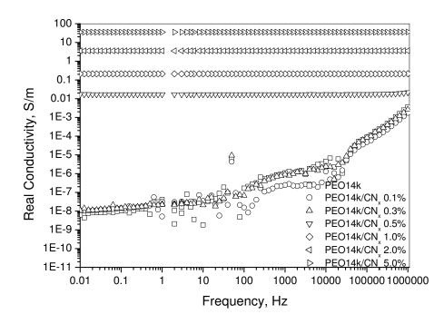
Fig. 7.43. Real conductivity of PEO14k/CN<sub>x</sub> nanocomposites vs. frequency at filler weight fractions of 0.1 to 5.0 wt% and applied voltage of 0.1 V.
