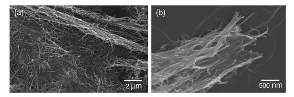
Fig. 5.22. STEM images of *in situ* polymerized  $PS-g-CN_x$  nanotube samples at magnifications (a) 32676X and (b) 8000X.
