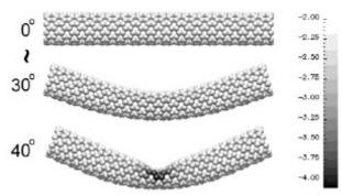
Fig. 2.2. The local chemical reactivity (hydrogenation energy) controlled by the carbon nanotube bending angle, that could be induced by mechanical deformations. The model considers only single bonds [19].
