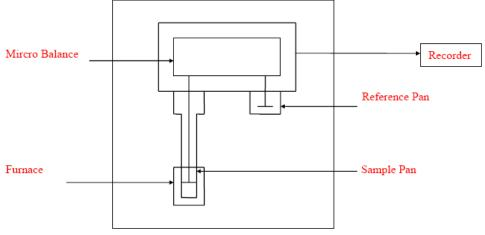
Fig. 4.13. Experimental set up of a Thermogravimeter.
