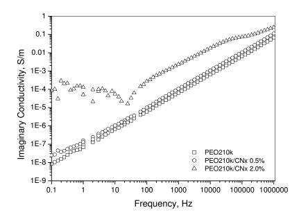
Fig. 7.39. Imaginary conductivity of PEO210k/CN<sub>x</sub> nanocomposites vs. frequency at filler weight fractions of 0.1 to 5.0 wt% and applied voltage of 0.1 V.
