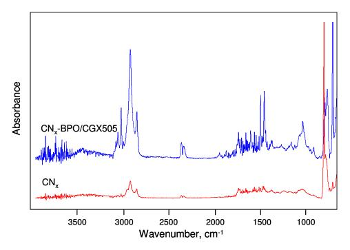
Fig. 5.13. FTIR spectra of CN<sub>x</sub> nanotubes and radical functionalized CN<sub>x</sub> nanotubes.
