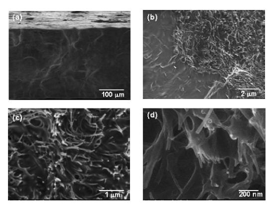
Fig. 6.16. SEM images of polymer nanocomposites of PEO and 2 wt% of PS-g-CN<sub>x</sub> nanotubes prepared by solution casting and film pressing.
