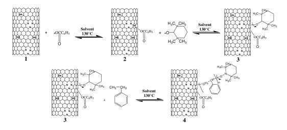
Fig. 5.1. Polymer brushes reaction scheme: functionalization of  $CN_x$  nanotubes (1) with the NMRP initiator (2) and controller (3), and synthesis of polymer brushes of polystyrene (4).
