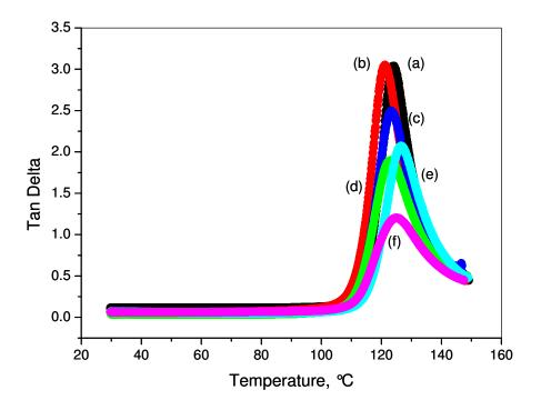
Fig. 7.12. Tan  $\delta$  of PS/CN<sub>x</sub> nanocomposites vs. temperature at filler weight fractions of (a) 0, (b) 0.3, (c) 0.5, (d) 1.0, (e) 2.0, and (f) 5.0 wt%.
