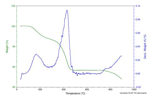
Fig. 5.7. Thermal degradation of radical functionalized reactor sample from the PPRs3, corresponding to F3 synthesized in benzene at 130°C using PR CGX 505 and low initiator concentration. The variables displayed are weight loss and its first derivative.
