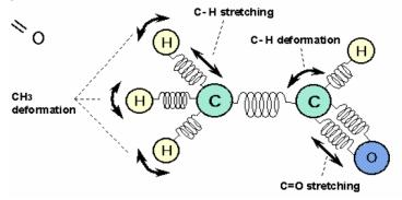
Fig. 4.11. Schematics of molecular vibration of polyatomic molecules.
