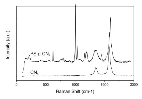
Fig. 5.28. Raman spectra of (a) raw  $CN_x$  nanotubes, and (b) *in situ* polymerized  $CN_x$  nanotubes (PSg-CN<sub>x</sub>) due to F3 reactor.
