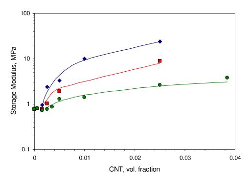
Fig. 7.20. Storage modulus of the PS/CNTs composites at several volume fractions of: ( $\diamond$ ) MWNT, ( $\Box$ ) CN<sub>x</sub> and ( $\circ$ ) PS-*g*-CN<sub>x</sub> filler. Lines show the fits obtained with the Percolation Model.
