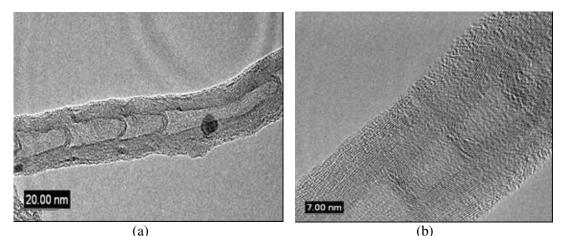
Fig. 5.8. HRTEM images of radical functionalized carbon nanotubes with BPO and TEMPO after dispersion by sonication in ethanol: (a) global view, (b) zoom.
