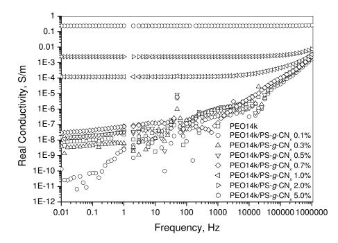
Fig. 7.45. Real conductivity of PEO14k/ PS-g-CN<sub>x</sub> nanocomposites vs. frequency at filler weight fractions of 0.1 to 5.0 wt% and applied voltage of 0.1 V.
