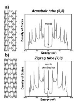
addition, bundles of SWNTs have shown metallic behavior with resistivities of  $0.34 \times 10^{-4}$  and  $1.0 \times 10^{-4}$  Ohm•cm [2].
