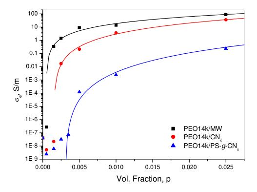
Fig. 7.24. Real part of the AC electrical conductivity at 1 Hz and 0.1 V for PEO14k/CNT at several filler contents. Comparison with statistical percolation theory (solid lines).
