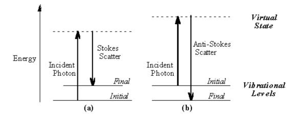
Fig. 4.10. Energy level diagram for Raman scattering: (a) Stokes Raman scattering, and (b) anti-Stokes Raman scattering [9].
