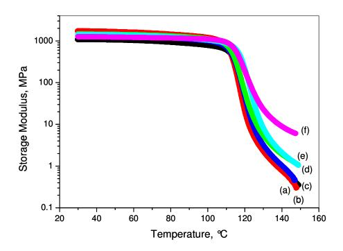
Fig. 7.11. Storage modulus of PS/CN<sub>x</sub> nanocomposites vs. temperature at filler weight fractions of (a) 0, (b) 0.3, (c) 0.5, (d) 1.0, (e) 2.0, and (f) 5.0 wt%.
