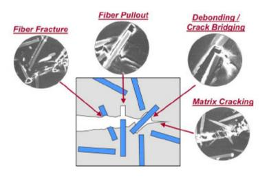
Fig. 3.2. Key mechanisms of energy dissipation have been identified in the fracture of short as well as continuous fiber-reinforced composites [1].
