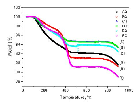
Fig. 5.6. Thermal degradation of radical functionalized reactor samples from the PPRs column 3, synthesized in benzene at 130°C using three nitroxides types: BPO/TEMPO ((a)A3 and (b)B3), BPO/OHTEMPO ((c) C3 and (d) D3) and PR CGX 505 ((e) E3 and (f) F3). A3, C3 and E3 consider high initiator concentration, whereas B3, D3 and F3 low initiator concentration.
