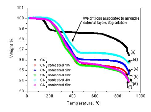
Fig. 5.2. Effect of sonication time in thermal degradation of CN<sub>x</sub> nanotubes: samples were sonicated (a) 0, (b) 1, (c) 2,(d) 3, (e) 4 and (f) 5 hr in xylene and dried in a vacuum oven for 15 hrs at 70-80°C. TGA in N from 20-900°C at 10°C/min.
