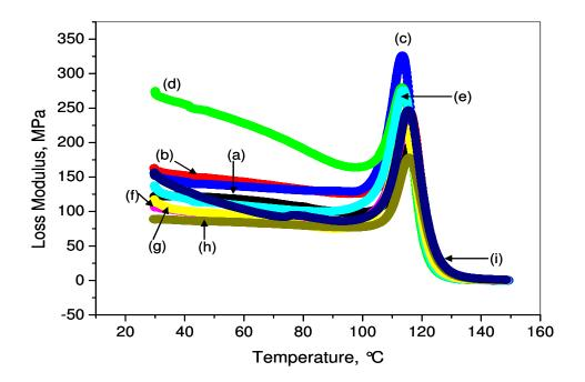
Fig. 7.36. Loss modulus of PS/PS-g-CN<sub>x</sub> nanocomposites vs. temperature at filler weight fractions of: (a) 0, (b) 0.1, (c) 0.3, (d) 0.5, (e) 0.7, (f) 1.0, (g) 2.0, (h) 5.0 and (i) 7.7 wt%.
