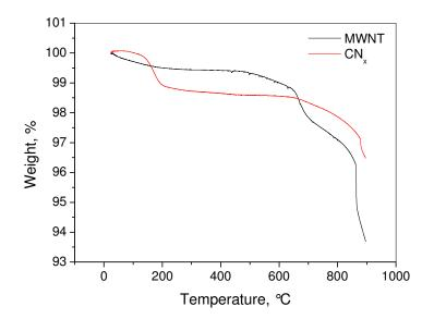
Fig. 4.5. Weight loss and degradation temperatures of as received carbon nanotubes: a) MWNTs, b) CN<sub>x</sub> nanotubes.
