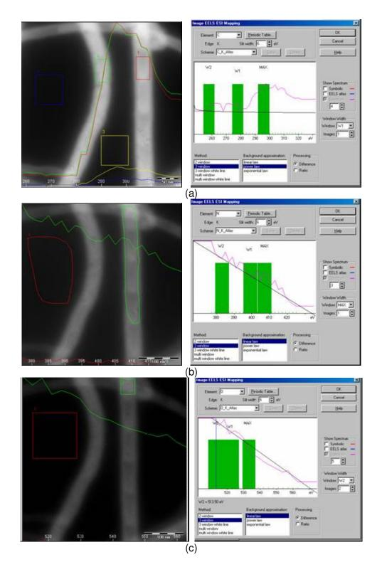
Fig. 5.27. EFTEM spectra extracted from the energy-filtered image series, and parameters used for the calculation of the elemental maps for the physical blend of PS and  $CN_x$  nanotubes (PS/CN<sub>x</sub>): (a) carbon map, (b) nitrogen map and (c) oxygen map.
