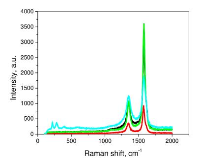
Fig. 4.4. D and G peak position and their relative intensities  $(I_D/I_G)$  of  $CN_x$  nanotubes Raman Spectra from samples of different batchs production.
