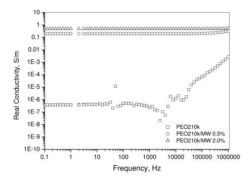
Fig. 7.21. Real conductivity of PEO210k/MWNT nanocomposites vs. frequency at filler weight fractions of 0.1 to 5.0 wt% and applied voltage of 0.1 V.
