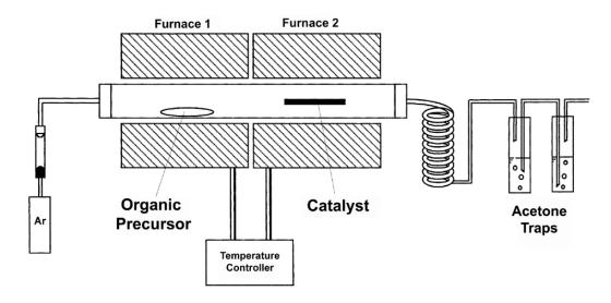
Fig. 1.7. Schematic diagram of the pyrolisis set up used for the synthesis of CNTs [2].
