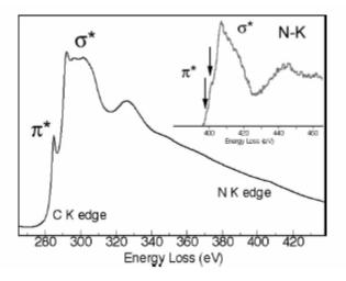
Fig. 1.12. EELS spectra of a CN<sub>x</sub> nanotube exhibiting K-shell ionization edges for C (~284.5 eV) and N (~400 eV). Inset shows (a) a sharp characteristic at ~401 eV corresponding to N bonded to C three C atoms within a hexagonal lattice, and (b) a weak shoulder at ~399 eV associated with pyridine-like N located in defective areas of the graphitic layers [54].
