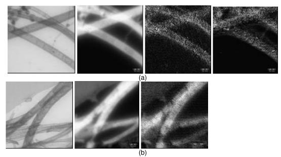
Fig. 5.9. Filtered images of (a) CN<sub>x</sub> nanotubes, and (b) CN<sub>x</sub>-RNO<sub>x</sub>. Each group of images is presented in the following order: zero loss, carbon, nitrogen and oxygen maps.
