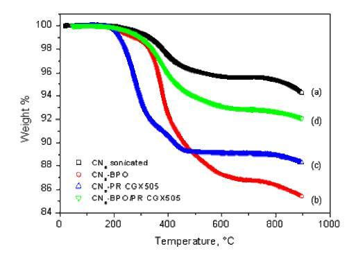
Fig. 5.12. Thermal degradation of  $CN_x$  nanotubes reacted with solutions of (b) BPO, (c) PR CGX505 and (d) BPO-PR CGX505 at same reaction conditions than F3 sample, but with twice of  $CN_x$  nanotubes.
