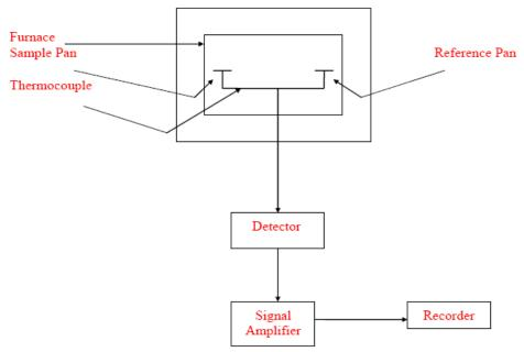
Fig. 4.15. Experimental device of a DS Calorimeter.
