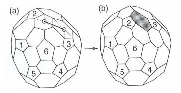
Fig. 1.17.  $C_2$  addition to a cap of nanotube. (a) Numbers from 1 to 6 indicate the position of the six pentagons on the hemispherical cap. If there is an addition of one  $C_2$  molecule, indicated by the open circles between 2 and 3, and if the new bonds denoted by dotted lines form, a new hexagon denoted in (b) by dark shading is obtained [3].
