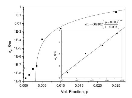
Fig. 7.49. Real part of the AC electrical conductivity at 1 Hz and applied voltage of 0.1 V for PEO14k/PS-g-CN<sub>x</sub> at several filler contents. Comparison with model (solid lines).
