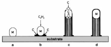
Fig. 1.19. Growth mechanism proposed by Baker *et al* for the formation of carbon nanotubes by pyrolisis. In this model, the carbon particles from the precursor, C, diffuse through metal catalyst, M, precipitating in the other side in the form of graphite. As can be seen, fiber formation take place in the substrate side [14].
