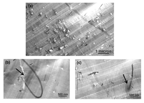
Fig. 6.4. TEM images of microtomed films of polymer nanocomposites of PS and 2 wt% of MWNT prepared by solution casting and high temperature pressing.
