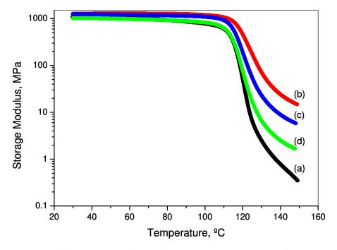
Fig. 7.17. Comparison of the Storage Modulus of (a) PS and PS-based composite with (b) MWNT, (c)  $CN_x$  and (d) PS-g- $CN_x$  nanotubes at a concentration of 5.0 wt%.
