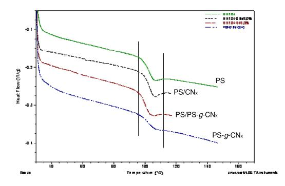
Fig. 6.2. Glass transition temperature of PS matrix, PS-grafted  $CN_x$  nanotube fillers alone (PSg-CN<sub>x</sub>) and the PS-based nanocomposites with either  $CN_x$  (PS/CN<sub>x</sub>), or PS-grafted  $CN_x$  fillers (PS/PS-g-CN<sub>x</sub>) at 5 wt%.
