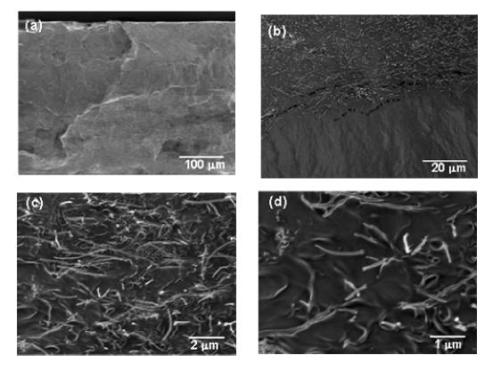
Fig. 6.13. SEM images of polymer nanocomposites of PEO and 2 wt% of MWNTs nanotubes prepared by solution casting and film pressing. Images (a) and (c) taken at normal scan and (b) and (d) at slow scan.
