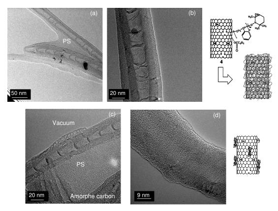
Fig. 5.23. HRTEM micrographs of the (a) and (b) *in situ* polymerized PS in the presence of  $CN_x$  nanotubes produced using the NMRP method, and (c) and (d) physical blend of PS with  $CN_x$  nanotubes.
