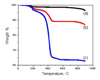
Fig. 5.20. Thermal degradation of reaction products of functionalized and polymer-grafted  $CN_x$  nanotubes (reactor F3): (a) as-produced  $CN_x$  nanotubes, (b) radical functionalized- $CN_x$  nanotubes ( $CN_x$ -RNO<sub>x</sub>), where the weight loss mainly corresponding to the BPO/PR CGX505 attachment, and (c) polymer-grafted- $CN_x$  (PS-*g*- $CN_x$ ) nanotubes where the weight loss corresponded to polymer attachment.
