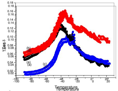
Fig. 7.26. Tan  $\delta$  of PEO/MWNT nanocomposite vs. temperature at filler weight fractions of (a) 0, (b) 0.5, and (c) 2.0 wt%.
