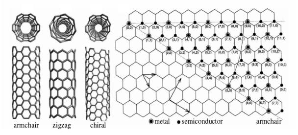
Fig. 1.3. Molecular models of SWNTs exhibiting different achiral and chiral conformations: (a) armchair, (b) zigzag and (c) chiral; (d) graphene sheet mathematic description, using chiral vector  $(C_h)$  with indexes (m,n) and unitary vectors  $(\mathbf{a}_1 \text{ and } \mathbf{a}_2)$ .
