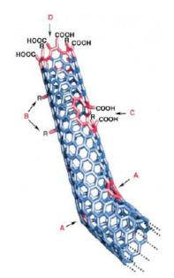
Fig. 2.3. The most common defect sites in SWNTs: A) Five or seven membered rings within the carbon framework (inducing bending); B) sp<sup>3</sup>-hybridized defects (R=H and OH); C) Carbon framework damage by oxidation, which leaves –COOH groups; D) Open ended SWNTs terminated with –COOH, or other terminal groups, such as -NO<sub>2</sub>, -OH, -H and =O [4].
