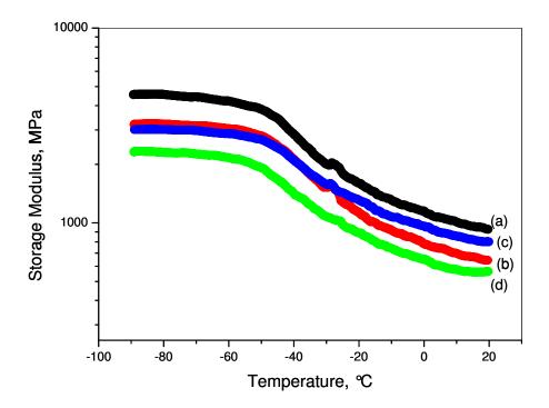
Fig. 7.27. Comparison of the Storage Modulus of (a) PEO and PEO-based composite with (b) MWNT, (c)  $CN_x$  and (d) PS-g-CN<sub>x</sub> nanotubes at a filler concentration of 2.0 wt%.
