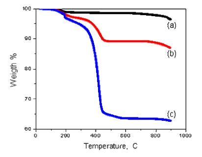
Fig. 5.21. Thermal degradation of reaction products of polymer-grafted CN<sub>x</sub> nanotubes at the conditions of reactor F3 using several radical functionalized samples: (a) CN<sub>x</sub>-BPO (CN<sub>x</sub>-R), (b) CN<sub>x</sub>-PR CGX505 (CN<sub>x</sub>-NO<sub>x</sub>), and (c) CN<sub>x</sub>-BPO/PR CGX505 (CN<sub>x</sub>-RNO<sub>x</sub>).
