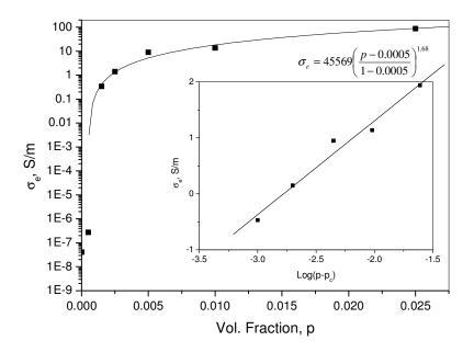
Fig. 7.47. Real part of the AC electrical conductivity at 1 Hz and applied voltage of 0.1 V for PEO14k/MWNT composites at several filler contents. Comparison with model (solid lines).
