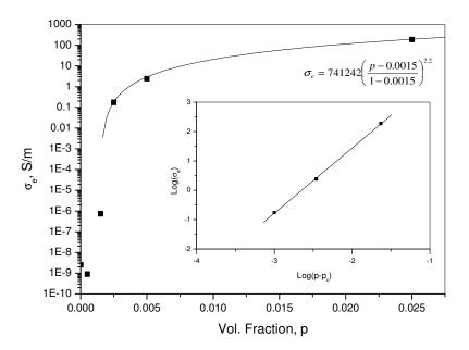
Fig. 7.33. Real part of the AC electrical conductivity at 1 Hz and 0.1 V for PS/CN<sub>x</sub> at several filler contents. Comparison with statistical percolation theory (solid lines).
