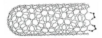
Fig. 1.18. Growth mechanism of carbon nanotubes at an open end by the absorption of  $C_2$  (dimmers) and  $C_3$  (trimers) [3].
