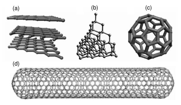
Fig. 1.1. Structure of crystalline carbon-based materials: (a) graphite, (b) diamond, (c) fullerene, and (d) SWNTs. (Molecular modeling images) [3].
