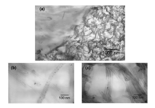
Fig. 6.15. TEM images of polymer nanocomposites of PEO and 2 wt% of  $CN_x$  nanotubes prepared by solution casting and film pressing.
