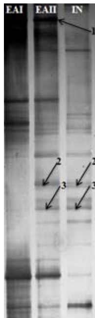
Fig. 3.6 DGGE profiles for archaea in experiment A. EAI: Experiment A stage I; EAII: Experiment A stage II; IN: Inoculum. Arrows and numbers indicate the successfully reamplified and sequenced bands.
