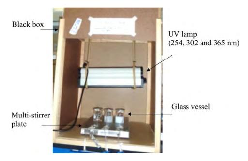
Figure 2.3. Photograph of the photoreactor 3UV.
