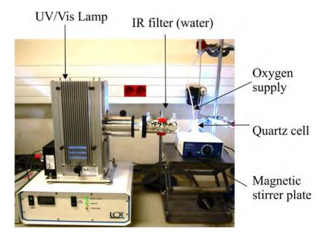
Figure 2.4. Photograph of the photoreactor Oriel.
