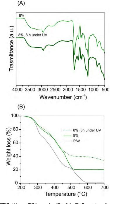
**Figure 4.10.** FTIR (A) and TGA spectra (B) of Ag/ZnO-poly(acrylic acid) composite under 8 h of UV irradiation exposure.
