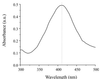
**Figure 2.A.** UV-Vis spectra of fresh solution of stabilized silver nanoparticles (OM20030601907)
