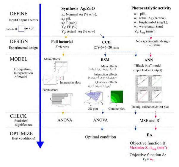
**Figure 6.3.** Scheme of the experimental design, model and optimization setting used to study the synthesis of Ag/ZnO photocatalyst and their photocatalytic behavior. The abbreviations FE: functionalization efficiency, CCD: central composite design, RSM: response surface methodology, ANN: artificial neural network, MSE: mean square error, EA: evolutionary algorithm.
