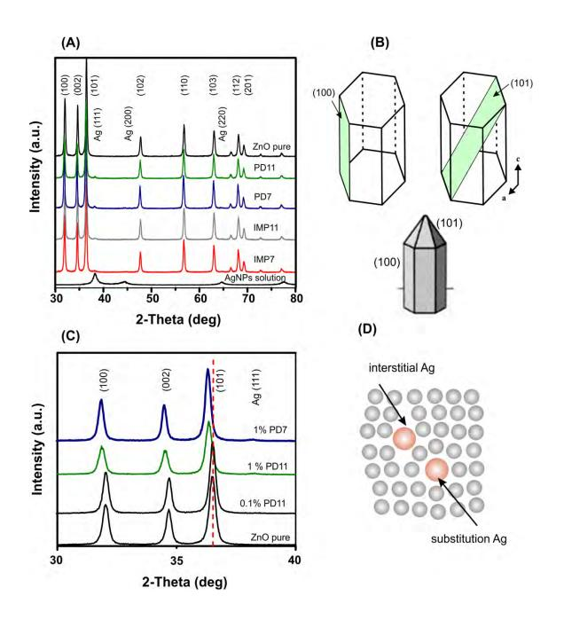
**Figure 3.3.** XRD pattern of 1%w/w Ag/ZnO obtained by photodeposition (PD) and impregnation (IMP) methods (A). ZnO unit cell showing (100) and (101) planes that lead the grow of nanorod with pyramidal tip (B). Zoom of Ag/ZnO XRD spectra showing the peaks shift (C) due to the insertion of Ag in ZnO crystallite (D).
