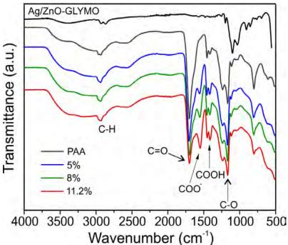
**Figure 4.3.** FTIR spectra of pure poly(acrylic acid) hydrogels and Ag/ZnO-poly(acrylic acid) nanocomposites. PAA: poly(acrylic acid).
