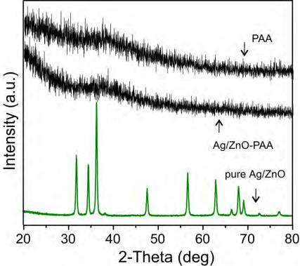
**Figure 4.7.** XRD pattern of poly(acrylic acid), Ag/ZnO and 8% Ag/ZnO-poly(acrylic acid) composites.
