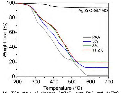
Figure 4.9. TGA curve of silanized Ag/ZnO, pure PAA and Ag/ZnO-PAA nanocomposites.
