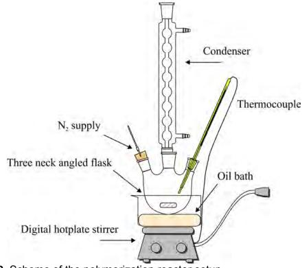
Figure 2.2. Scheme of the polymerization reactor setup.
