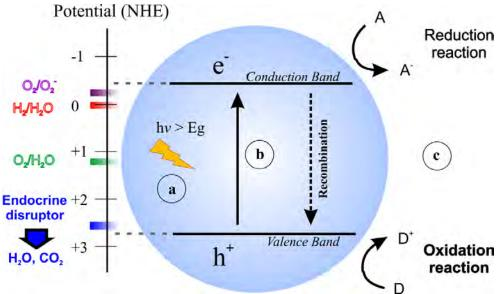
**Figure 1.2.** Schematic representation of the photocatalytic mechanism of ZnO where a) the photon energy greater than the bandgap energy is adsorbed by ZnO and generates electron-hole pairs, b) the photoexcited charge carriers spate and migrate to the surface, and c) adsorbed species are reduced and oxidized by the photogenerated electrons and holes, respectively. (A/A<sup>-</sup>: acceptor species, D/D<sup>+</sup> donor species).
