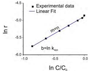
**Figure 5.1.** Linear plot Y=mx + b to obtain the kinetics parameters (k<sub>app</sub> and n).
