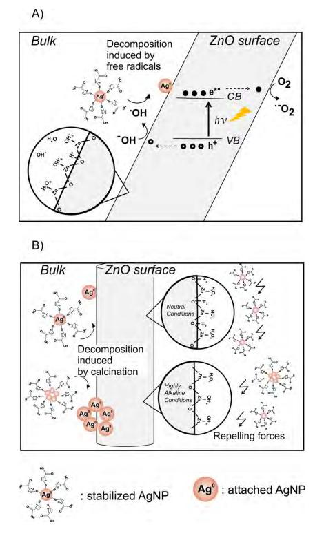
**Figure 3.2.** Mechanism for functionalization of ZnO with silver nanoparticles by photodeposition method (A) and impregnation method (B).
