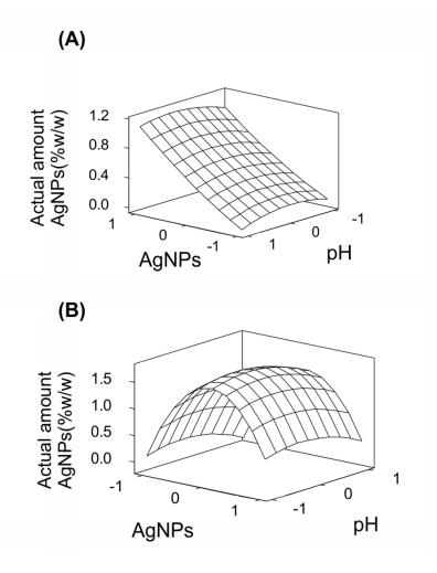
**Figure 6.5.** 3D surface plot of the effect of actual amount AgNPs and pH on the response of the RSM model of the functionalization of ZnO by the (A) photodeposition and (B) impregnation method.
