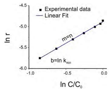
**Figure 6.2.** Linear plot Y=mx + b to obtain the kinetics parameters (k<sub>app</sub> and n).
