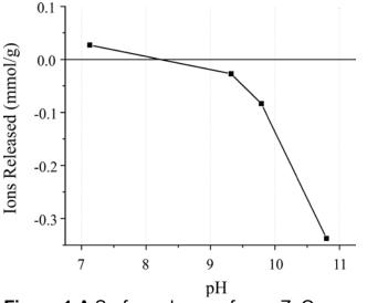
Figure 1.A Surface charge of pure ZnO.
