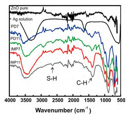
Figure 3.7. FTIR spectra of pure ZnO, AgNPs and 1%w/w Ag/ZnO.
