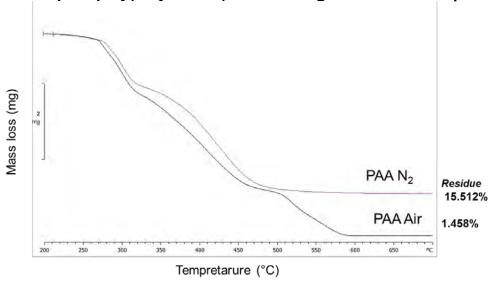
TGA of pure poly(acrylic acid) under nitrogen and air atmosphere
