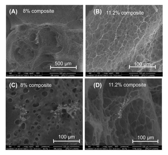
**Figure 4.5.** SEM images of swollen Ag/ZnO-poly(acrylic acid) nanocomposites. Low magnification (A, B) and high magnification (C, D).
