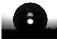
**Figure 4.8.** Images of water droplet on (A) 8% Ag/ZnO-poly(acrylic acid) nanocomposite (contact angle=  $117.8\pm2.51^{\circ}$ ) and (B) pure ZnO photocatalyst (contact angle=  $135\pm3.65^{\circ}$ ) placed on a glass slide.
