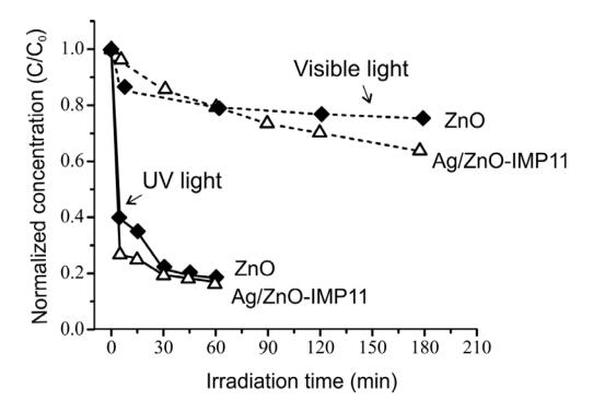
**Figure 5.10.** Normalized concentration of triclosan in function of time using pure ZnO and Ag/ZnO photocatalysts (test conditions: triclosan=20 mg/L,  $\lambda$ =302 nm, pH=8.6, photocatalyst= 0.5 g/L).
