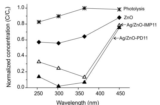
**Figure 5.4.** Normalized concentration of bisphenol-A at different wavelength using ZnO and Ag/ZnO photocatalyst (test conditions: BPA=10 mg/L, photocatalyst= 1 g/L, pH=10.5, reaction time of 120 min for  $\lambda$ =254, 302, 365 nm, and 180 min for  $\lambda$ >450 nm).
