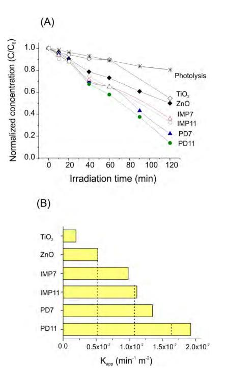
**Figure 5.2.** (A) Photocatalytic activity of 1%w/w Ag/ZnO and (B) surface area normalized rate constant of bisphenol-A degradation (test conditions: BPA=10 mg/L, photocatalyst= 1 g/L, pH=10.5, reaction time of 120 min for  $\lambda$ =302 nm).
