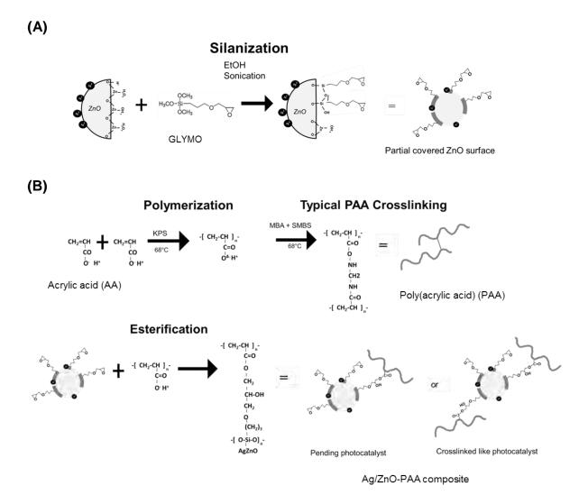
**Figure 4.1.** Representation of the mechanism of Ag/ZnO silanization with GLYMO (A) and the Ag/ZnO-poly(acrylic acid) composite synthesis (B).
