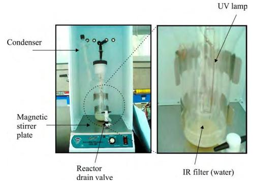
**Figure 2.1.** Photograph of the photoreactor Q200 for the functionalization of ZnO by the photodeposition method.
