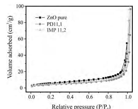
**Figure 3.5.** N<sub>2</sub> adsorption-desorption isotherm of 1% w/w Ag/ZnO photocatalyst prepared by the photodeposition (PD) and impregnation (IMP) method.
