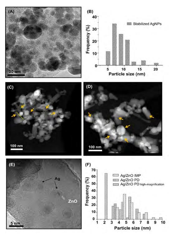
**Figure 3.4.** TEM images of stabilized AgNPs (A, B) and 1%w/w Ag/ZnO photocatalyst prepared by the photodeposition method (C, E: high-magnification) and impregnation method (D). Frequency histograms of AgNPs size before (B, n=106) and after (F, n=40) functionalization of ZnO.
