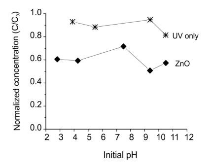
**Figure 5.5.** Normalized concentration of bisphenol-A at different pH using ZnO (test conditions: BPA=10 mg/L, photocatalyst= 1 g/L,  $\lambda$ =302 nm, reaction time=120 min).
