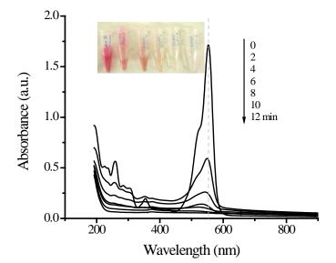
**Figure 2.C.** Evolution of the UV-Vis spectra of rhodamine-B degradation using Ag/ZnO-PD11 photocatalyst under UV light (test conditions: rhodamine-B =47 mg/L, photocatalyst= 1 g/L,  $\lambda$ =254 nm). Photograph of rhodamine-B discoloration in function of time.
