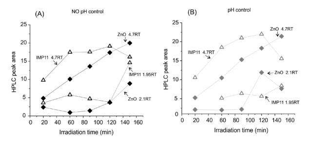
**Figure 5.8.** Time evolution of byproducts profile in time detected by HPLC during bisphenol-A degradation under uncontrolled pH (A) and controlled pH (B). RT: retention time (min) recorded in the chromatogram (see Appendix C). Test conditions: BPA=10 mg/L, photocatalyst= 1 g/L,  $\lambda$ =302 nm, pH=10.5.
