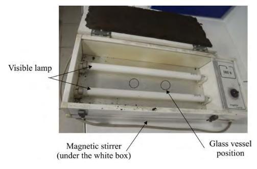
Figure 2.5. Photograph of the photoreactor Vilber.
