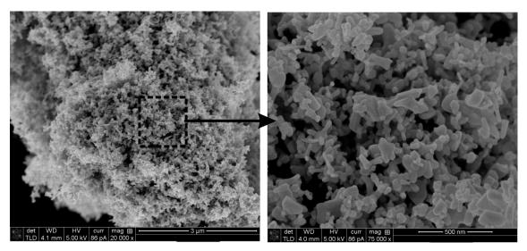
**Figure 1.5.** SEM photograph of the commercial ZnO nanoparticles (VP AdNano ZnO 20DW, Degussa Co.) used in this thesis. The different morphologies include rods, tetrapods with both pyramidal and round tips.
