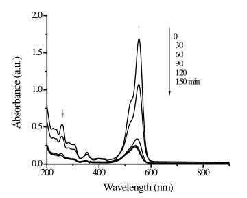
**Figure 3.C.** Evolution of the UV-Vis spectra of rhodamine-B degradation using Ag/ZnO-PD11 photocatalyst under Visible light (test conditions: rhodamine-B =47 mg/L, photocatalyst= 1 g/L,  $\lambda$ >455 nm).
