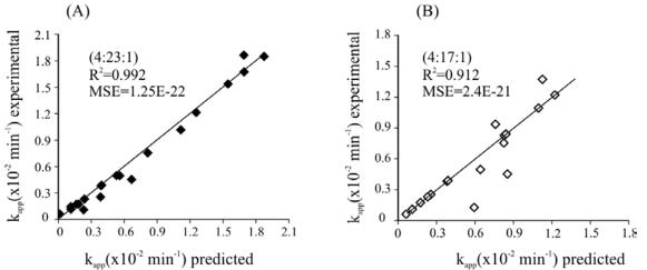
**Figure 6.7** Plot of the experimental data against predicted data by ANN model for apparent rate constant ( $k_{app}$ ) of the bisphenol-A degradation using Ag/ZnO photocatalysts obtained by the (A) photodeposition and (B) impregnation methods.
