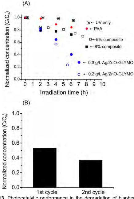
**Figure 5.13.** Photocatalytic performance in the degradation of bisphenol-A using pure Ag/ZnO-GLYMO photocatalyst and Ag/ZnO-poly(acrylic acid) composites (A) and overall photodegradation performance after two cycles of 8 h (B) (test conditions: bisphenol-A =10 mg/L,  $\lambda$ =365 nm, pH=10.5).
