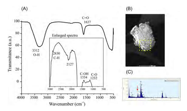
**Figure 3.6.** FTIR spectra (A) and TEM image (B) of stabilized AgNPs. EDX elemental analysis (C) corresponds to the squared area in B.
