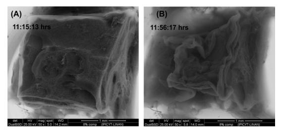
**Figure 1.B** Low vacuum ESEM images of 8% Ag/ZnO-poly(acrylic acid) composite in taken in different times. Note the porosity of the fresh swollen (A) and dehydrated-collapsed sample (B). The time-window of the analysis is 40 min.
