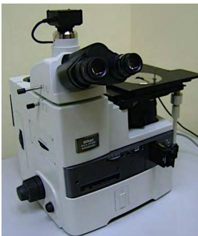
Figura 2.6 Microscopio NIKON MA 200.
