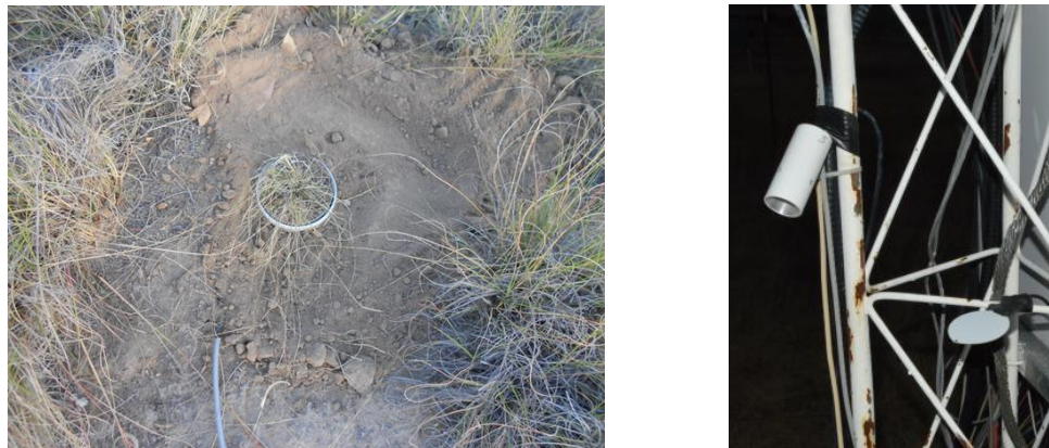
Figure 2. A microlysimeter and leaf wetness sensor (LWS) installed in the study area.
