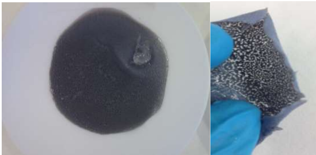
Figure 27. Images of the nano-ZnO/GO/PVA polymeric composite and its surface characteristics.
