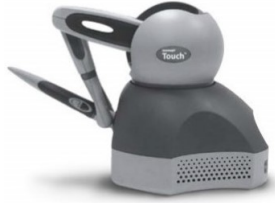
Figure 1.3: 3-DOF Geometric Touch Haptic Device at Universidad de Guadalajara .
