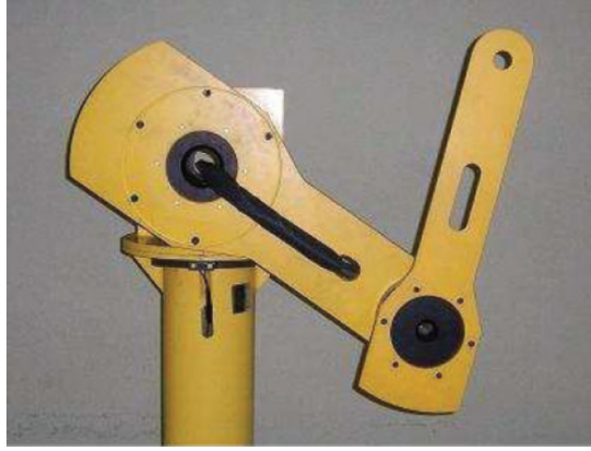
Figure 1.1: 2-DOF robot manipulator at Instituto Tecnológico de la Laguna .
