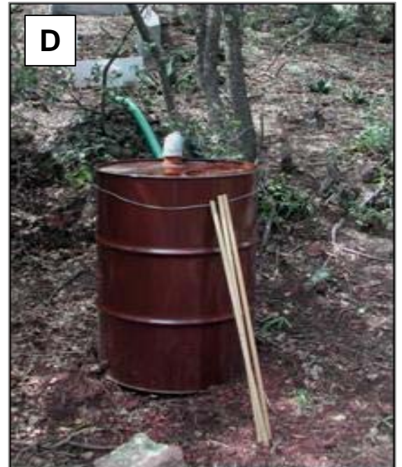
Photo1.2 Experimental set-up for monitoring stemflow (A and B) and runoff (C and D)
