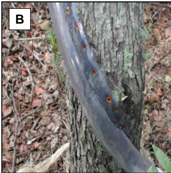
Photo1.2 Experimental set-up for monitoring stemflow (A and B) and runoff (C and D)
