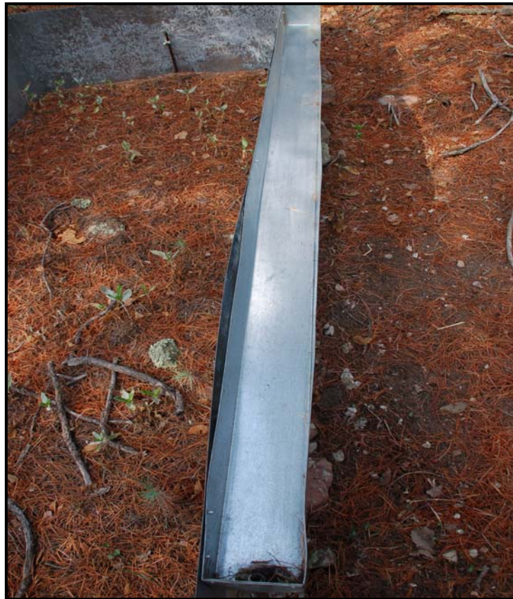
Photo1.3 Experimental set-up for monitoring throughfall
