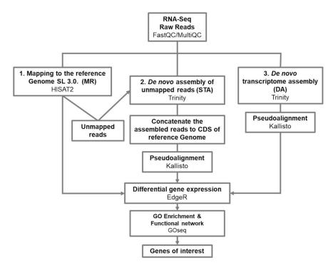
**Figure 2.** RNA-Seq data processing pipelines. The scheme summarizes the three strategies for data analysis: direct mapping to the reference genome of *Solanum lycopersicum* SL3.0, MR; (left), de novo assembly of unmapped reads, STA; (center), and de novo transcriptome assembly, DA (right). Processes and strategies are shown in bold and bioinformatic packages used for those processes are represented in light font.
