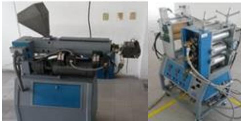
Figure 30. Extrusion equipment for film formation.
